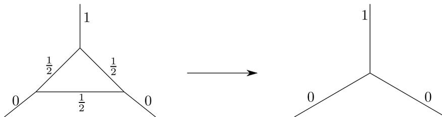
FIG. 12. Gauss constraint violations under coarse graining (for  $SU(2)$ ): we can define an effective vertex by summing over the  $SU(2)$  representations associated to the inner edges. The configuration on the left is allowed by the coupling rules, thus the effective vertex on the right is allowed. However, this configuration is forbidden by  $SU(2)$  coupling rules.
