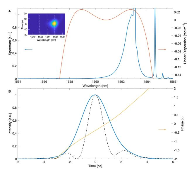
**Fig. 3.** Analysis of individual soliton atoms of the molecule. (A) Measured output spectrum (blue curve) and net linear dispersion relation (orange curve). The inset shows the measured spectrogram with white dashed lines denoting the locations of the peaks and central frequency in the dispersion relation. (B) Retrieved temporal intensity (blue curve) and temporal phase (yellow curve) of single-peaked spectrum and retrieved temporal intensity of double-peaked spectrum (dashed black curve).
