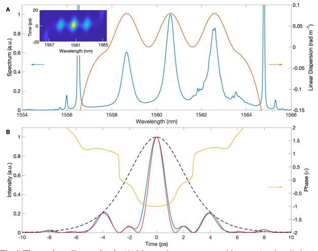
**Fig. 4. Three color soliton molecule.** (**A**) Measured output spectrum (blue curve) and applied netcavity linear dispersion relation (orange curve). The inset shows the measured spectrogram. (**B**) Retrieved temporal intensity (blue curve), predicted temporal intensity (red curve), hyperbolic secant shaped envelope (dashed black curve) and retrieved temporal phase (yellow curve).
