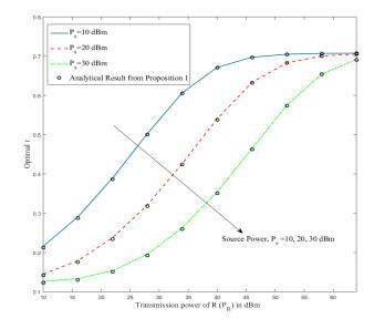
Fig. 2. Plot of instantaneous secrecy capacity using (9) for various values of  $P_R$  and  $P_S$ .  $d_{SR} = d_{SJ} = d_{RD} = 20m$ ,  $d_{RE} = 30m$ ,  $d_{JE} = 10m$ ,  $\alpha = 3$ ,  $\sigma_n^2 = -80$  dBm and N = 500.  $X_{RE} = X_{RD} = 1$ ,  $X_{JE} = 0.82$ ,  $\mathbf{h}_{SR}$  and  $\mathbf{h}_{SJ}$  are generated in MATLAB in same sequence with rng (100).
