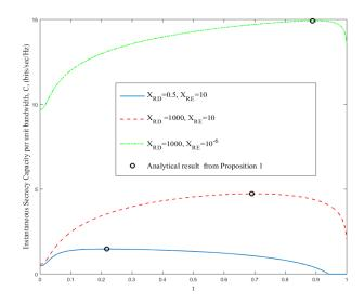
Fig. 1. Plot of instantaneous secrecy capacity using (9) for various values of  $t. d_{SR} = d_{SJ} = d_{RD} = d_{RE} = d_{JE} = 100$ m,  $\alpha = 3$ ,  $P_S = P_R = 30$  dBm,  $\sigma_n^2 = -110$  dBm and N = 200.  $X_{JE} = 1$ ,  $\mathbf{h}_{SR}$  and  $\mathbf{h}_{SJ}$  are generated in MATLAB in same sequence with rng (10).
