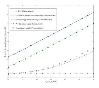
Fig. 3. Plot of ergodic secrecy capacity through simulations and ESR using (12) for various values of  $P_R$  and  $P_S$ .  $d_{SR} = d_{SJ} = 50m$ ,  $d_{RD} = 30m$ ,  $d_{RE} = 60m$ ,  $d_{JE} = 40m$ ,  $\alpha = 2.7$ ,  $\sigma_n^2 = -80$  dBm and N = 300.
