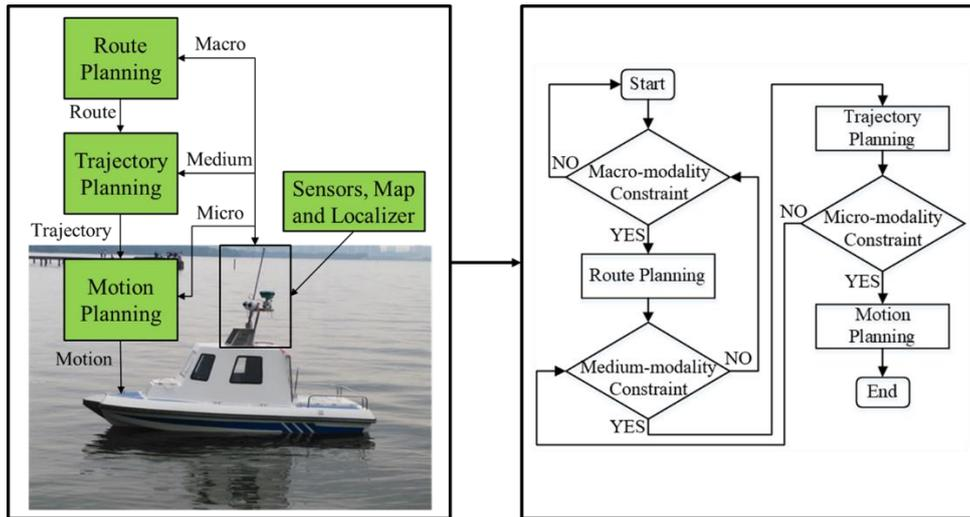
Figure 1 USV Path Planning based on multi-modality constraint
