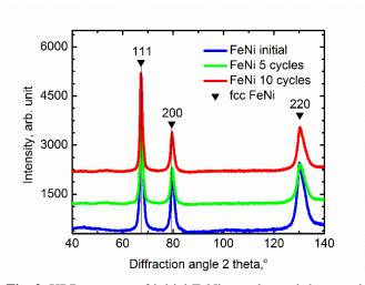
**Fig. 2.** XRD patterns of initial FeNi samples and the samples subjected to 5 and 10 cycles of treatments.
