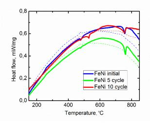
**Fig. 3.** DSC curves of initial FeNi samples and the samples subjected to 5 and 10 cycles of treatments upon heating (solid lines) and cooling (dashed lines).
