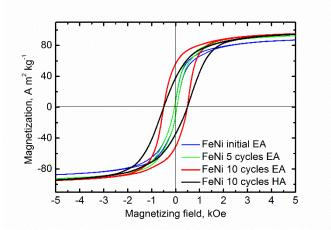
**Fig. 4.** Magnetization curves of initial FeNi samples and the samples subjected to 5 and 10 cycles of treatments.
