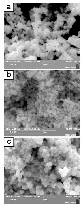
**Fig. 1**. SEM images of FeNi nanopowders: a – initial sample, b – after 5 cycles and c – after 10 cycles of the treatments.
