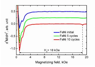
**Fig. 5.** SPD curves of initial FeNi samples and the samples subjected to 5 and 10 cycles of treatments.
