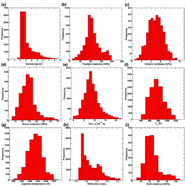
**Figure 1. Dataset visualization.** Distribution of the properties, namely, (a) density, (b) Young's modulus, (c) hardness, (d) shear modulus, (e) thermal expansion coefficient (TEC), (f) glass transition temperature (T<sub>g</sub>), (g) liquidus temperature, (h) refractive index, and (i) bulk modulus, in the glass dataset used for training the GPR model.
