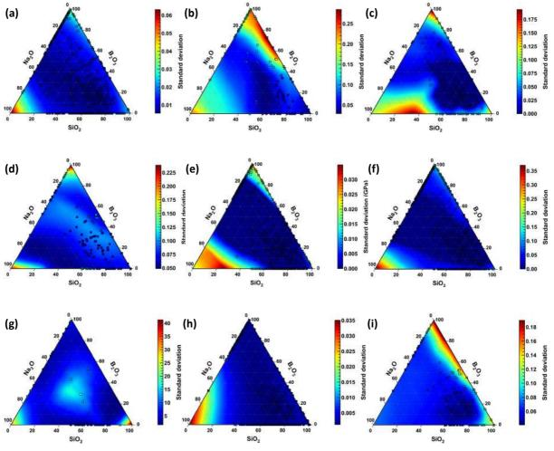
**Figure 3. Standard deviation for predicted values using KISS-GP.** Standard deviation predicted by the trained GPR models of (a) density, (b) Young's modulus, (c) hardness, (d) shear modulus, (e) thermal expansion coefficient (TEC), (f) glass transition temperature (T<sub>g</sub>), (g) liquidus temperature, (h) refractive index, and (i) bulk modulus for sodium borosilicate glasses. Experimental values are marked using back squares.
