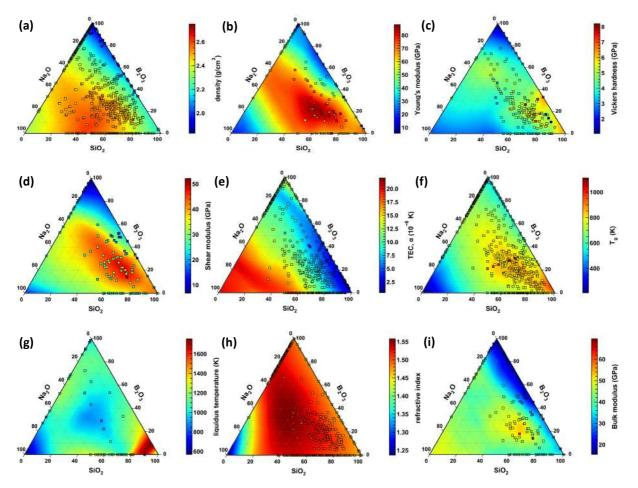
**Figure S3.** Predicted values of (a) density, (b) Young's modulus, (c) hardness, (d) shear modulus, (e) thermal expansion coefficient (TEC), (f) glass transition temperature (T<sub>g</sub>), (g) liquidus temperature, (h) refractive index, and (i) bulk modulus by the trained GPR models for sodium borosilicate glasses. Experimental values are marked using back squares.
