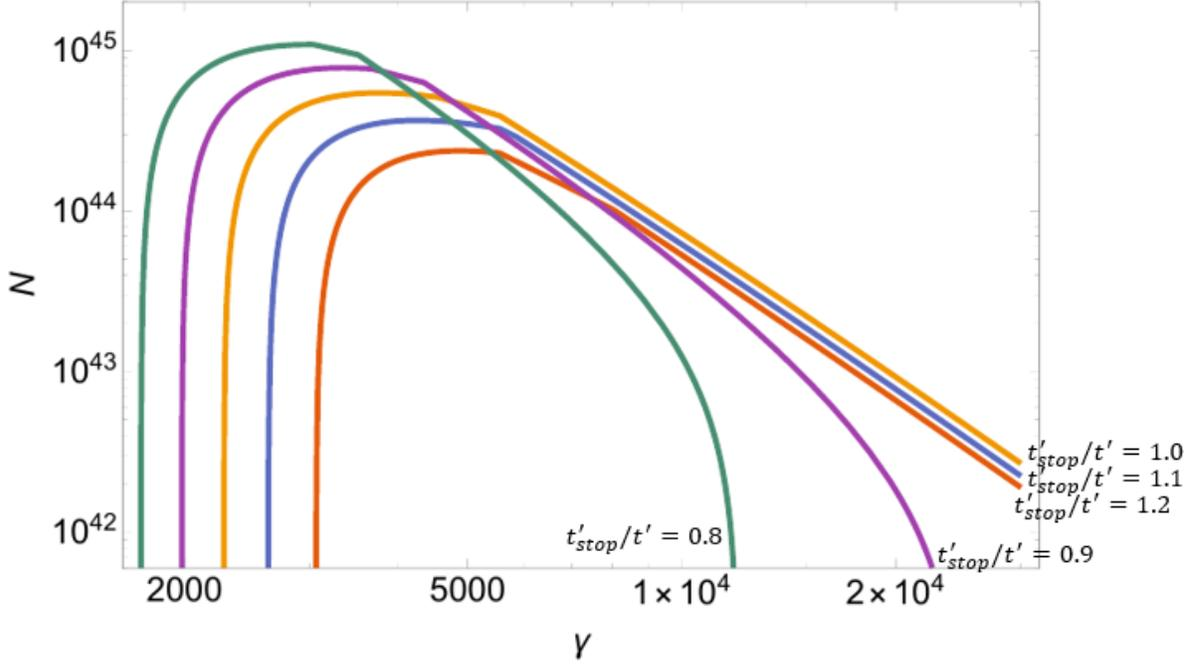
Fig. 3.— Evolution of the distribution function. Here we take account the effect of radiation loss and adiabatic expansion. In our calculation, the Lorentz factor of RS  $\gamma_{RS} = 90$ , and the injection is stopped at time  $t'_{\text{stop}} = 1.5 \times 10^5 \text{s}$ ,  $\gamma_{\text{min}} = \gamma_w/\gamma_{RS} = 5556$ , initial magnetic field  $B_0 = 2.1 \text{G}$ . The times are measured in fluid frame at  $t'_{\text{stop}}/t' = 1.2, 1.1, 1.0, 0.9, 0.8$  from red to green curves.
