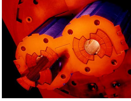
Fig. 9: Superconducting dipole magnets of the LHC.
