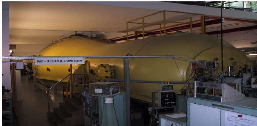
Fig. 4: A typical example of a Tandem-van-de-Graff Accelerator. These are very reliable machines for precision measurements in atom and nuclear physics. (Photo: Max Planck Institute for Nuclear Physics, Heidelberg)
