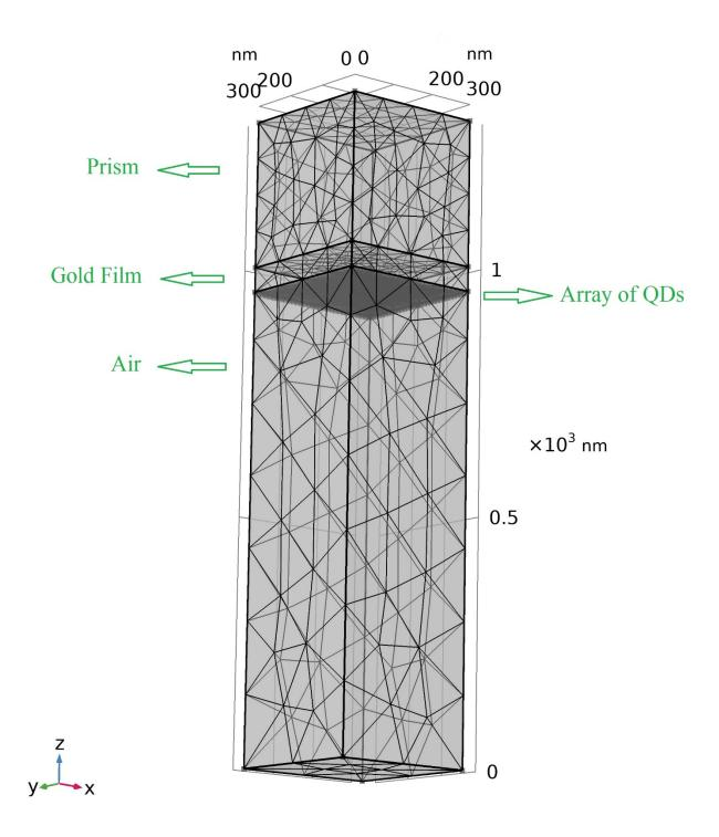
Figure 11. Meshed structure of SPPs-QDs coupling
