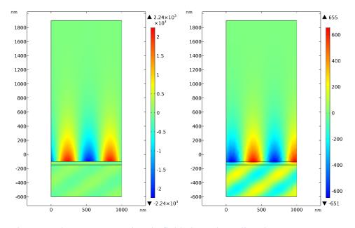
Figure 9. The evanescent electric field along the z-direction
