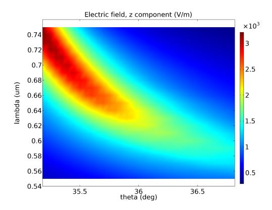
Figure 10. Maximum E-field magnitude on the surface of the 48 nm gold film
