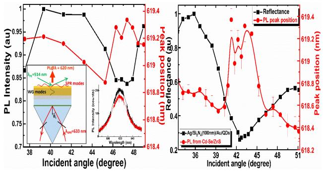
Figure 7 (a). Schematic of the prism setup to create SPR and PL emission, The PL spectra show SPR-induced quenching.
