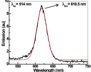
Figure 6. PL spectrum of QDs pumped by 514 nm green laser.
