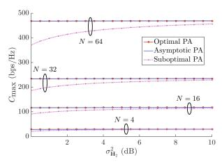
Figure 4: Sum-capacity vs channel gain of weak user
