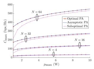
Figure 2: Sum-capacity vs total transmission power
