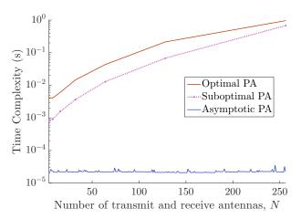
Figure 5: Time complexity of power allocation algorithms
