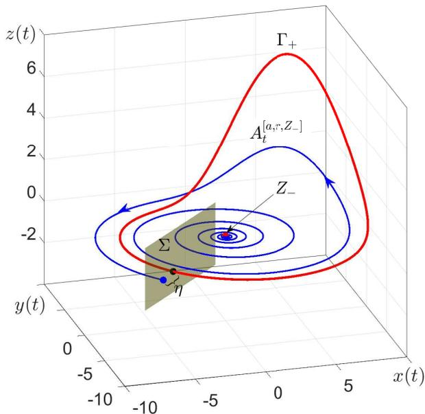
Figure 4: A schematic diagram showing the shooting method we use to find the connection between  $Z_-$  and  $\Gamma_+$  for (5), see Appendix A for animated version of this figure.
