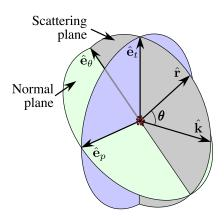
FIG. 1. Scattering geometry.  $\hat{\mathbf{k}}$  indicates the laser photon propagation direction.  $\hat{\mathbf{r}}$  indicates the observation direction.  $\hat{\mathbf{e}}_{p}$ ,  $\hat{\mathbf{e}}_{t}$  and  $\hat{\mathbf{e}}_{\theta}$  are linear polarization vectors.
