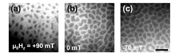
Figure 2: MTXM images of the skyrmion phase in the [Co (0.7 nm)/ Ni (0.5 nm)/ Pt (0.7 nm)]<sub>20</sub> sample as the out-of-plane field strength was varied. Before imaging, the stripe-to-skyrmion transformation was accomplished by applying a 60- $\mu$ s current pulse of density 1.7 x 10<sup>10</sup> A/m<sup>2</sup> in a field of  $\mu_0 H_z = +190$  mT. (bar = 500 nm)
