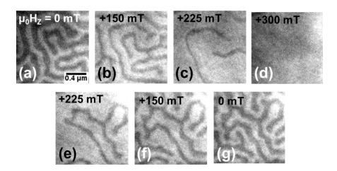
Supplemental Figure S1: Magnetic transmission X-ray microscopy (MTXM) images of the magnetic domain morphology as an out-of-plane magnetic field ( $\mu_0 H_Z$ ) was swept from zero towards positive saturation then back to zero in a Ta (2)/ Pt (5)/[Co (0.7)/ Ni (0.5)/Pt (0.7)]<sub>20</sub>/ Ta (5) (thicknesses in nm) sample.
