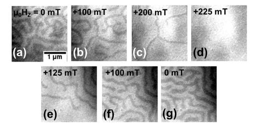
Supplemental Figure S6: MTXM images of the magnetic domain morphology as an out-of-plane magnetic field ( $\mu_0H_Z$ ) was swept from zero towards positive saturation then back to zero in the Ta (2)/ Pt (5)/[Co (0.7)/Tb (0.4)/Ni (0.5)/Pt (0.7)]<sub>20</sub>/ Ta (5) (thicknesses in nm) sample.
