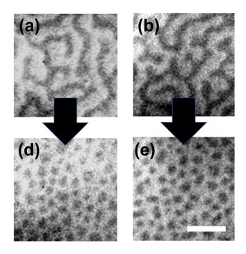
Supplemental Figure S8: MTXM images illustrating the effect of applying a  $\tau=50~\mu s$ -long current pulse with density 1.7 x  $10^{10}~A/m^2$  on the domain morphology of the (a) Ta (2)/Pt (5)/[Co (0.7)/ Ni (0.5)/Pt (0.7)]<sub>20</sub>/Ta (5) sample and the (b) Ta (2)/ Pt (5)/[Co (0.7)/ Ni (0.5)/Pt (0.7)]<sub>20</sub>/ Pt (5) (thicknesses in nm) samples in an applied magnetic field of +50 mT. (scale bar = 400 nm)
