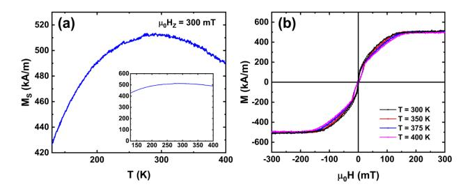
Supplemental Figure S5: (a) The saturation magnetization  $M_S$  as a function of temperature, and (b) in-plane hysteresis loops at selected temperatures of an unpatterned Ta (2)/ Pt (5)/[Co (0.7)/Tb (0.4)/Ni (0.5)/Pt (0.7)]<sub>20</sub>/ Ta (5) (thicknesses in nm) sample, determined using vibrating sample magnetometry.
