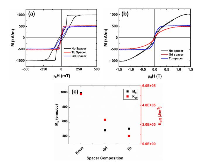
Supplemental Figure S4: (a) Out-of-plane and (b) in-plane vibrating sample magnetometry characterization of the room temperature magnetic properties of the Ta (2)/Pt (5)/[Co (0.7)/Spacer (0.4)/Ni (0.5)/Pt (0.7)]<sub>20</sub>/ Ta (5) (thicknesses in nm) samples. (c) Saturation magnetization ( $M_S$ ) and effective perpendicular anisotropy energy density ( $K_{eff}$ ) of the samples determined from (a) and (b).
