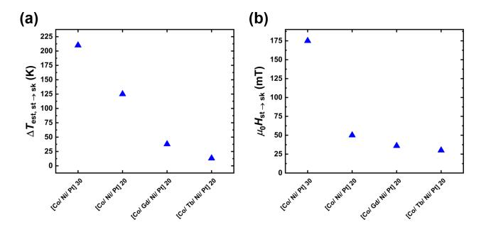
Figure 7: (a) The experimentally estimated temperature change due to Joule heating ( $\Delta T_{\rm est, \ st \rightarrow sk}$ ) and (b) perpendicular field ( $\mu_0 H_{\rm st \rightarrow sk}$ ) necessary to initiate a complete stripe-to-skyrmion transformation in the [Co/ Ni/ Pt]-based samples reported here. Data corresponds to the necessary electrical pulse characteristics at the lowest possible magnetic field.
