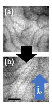
Supplemental Figure S7: MTXM images depicting the change in domain morphology of the Ta (2)/ Pt (5)/[Co (0.7)/Tb (0.4)/Ni (0.5)/Pt (0.7)]<sub>20</sub>/ Ta (5) (thicknesses in nm) sample before (a) and after (b) a 200- $\mu$ s pulse of current density 2.4 x 10<sup>9</sup> A/m<sup>2</sup> was applied in an applied magnetic field of + 40 mT. The blue arrow indicates the electron flow direction  $j_e$ . (bar = 500 nm)
