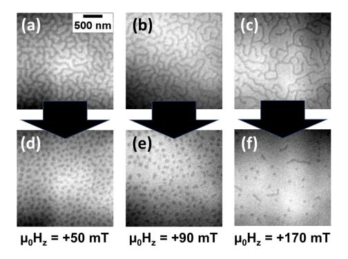
Supplemental Figure S3: MTXM images illustrating the effect of applying a  $\tau = 100$  µs-long current pulse with density 1.7 x  $10^{10}$  A/m² on the domain morphology of a Ta (2)/ Pt (5)/[Co (0.7)/ Ni (0.5)/Pt (0.7)]<sub>20</sub>/ Ta (5) (thicknesses in nm) sample patterned into a wire for applied magnetic fields of  $\mu_0 H_z = +50$  (a, d), +90 (b, e), and +120 mT (c, f).
