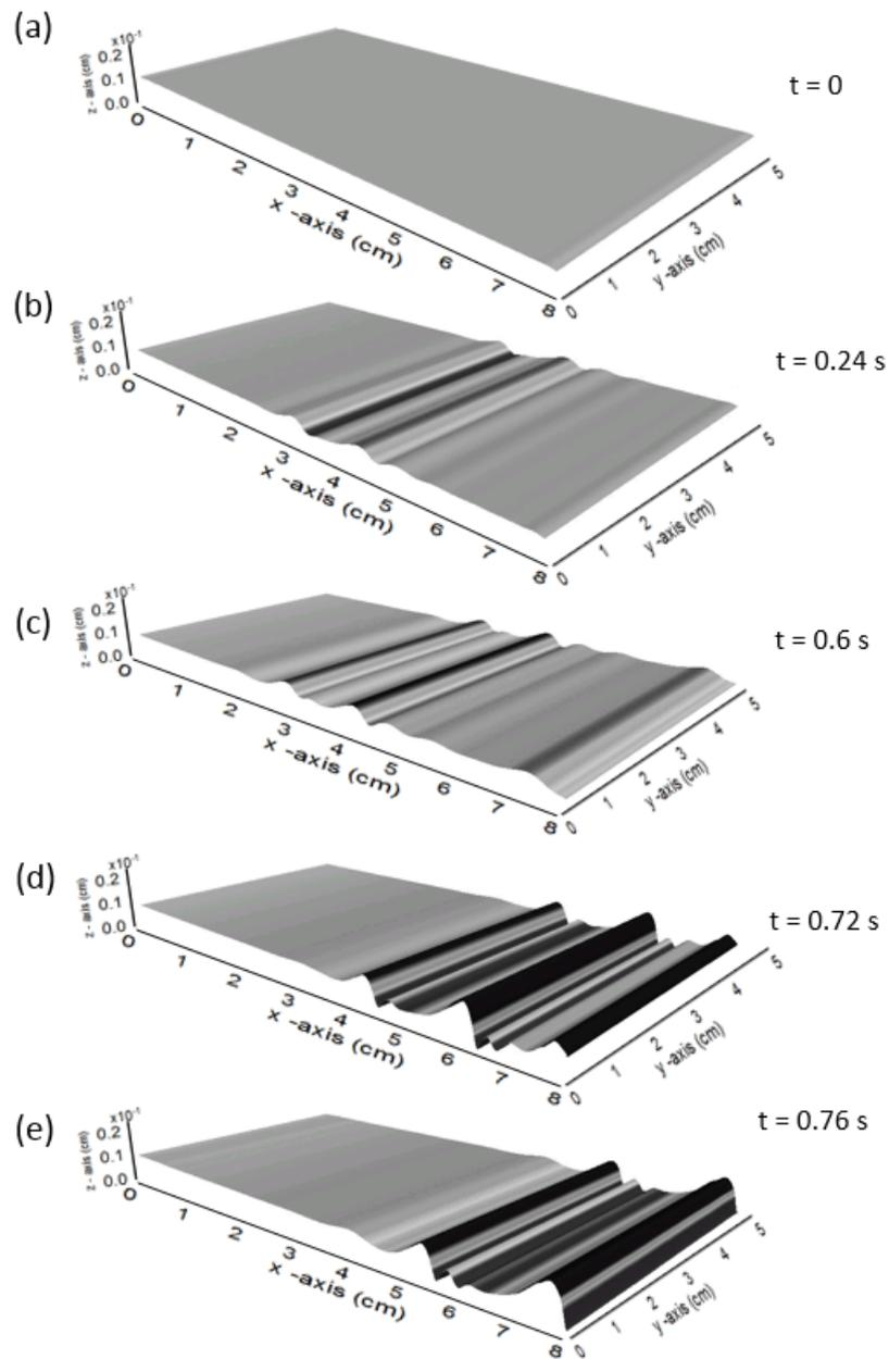
**Fig. 9** Interface profile for the propagation of gamma II wave family in three dimensions (code Blue). Simulation parameters are  $Re\ 62$ ,  $\beta = 90$ ,  $F = 15 \text{ Hz}$ . The interface height has been magnified to clearly reveal the wave propagation. The computed wave speed is  $0.233 \text{ m/s}$
