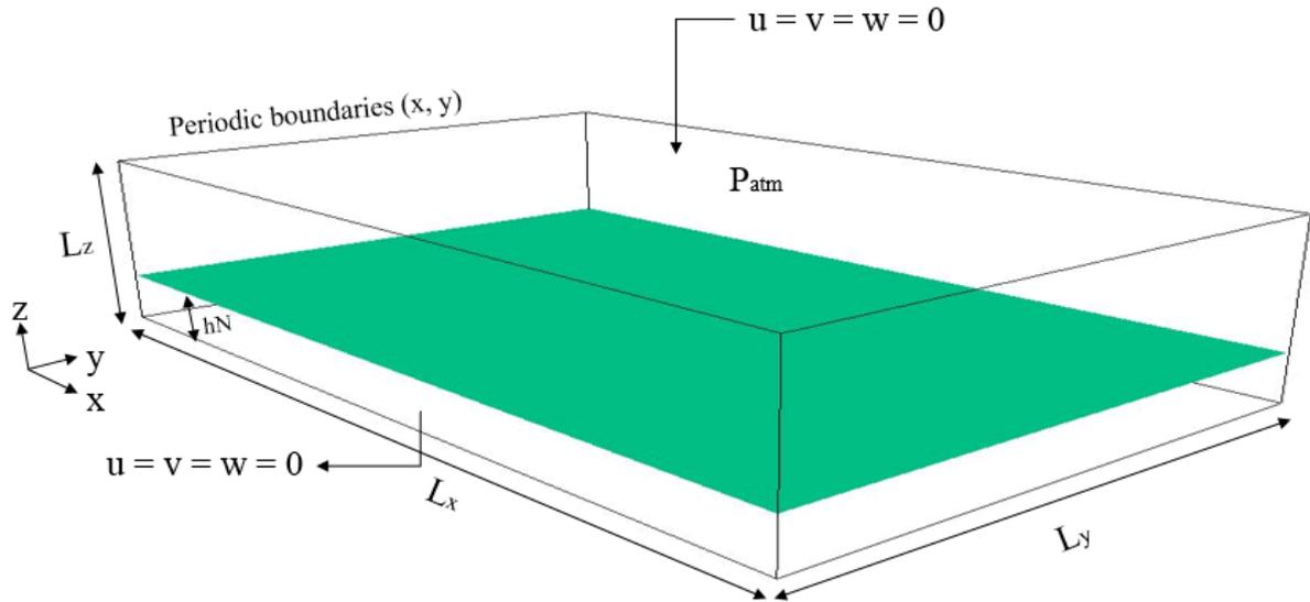
**Fig. 1** The computational domain of the numerical set-up
