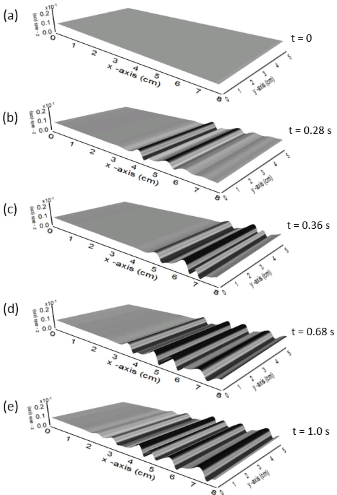
**Fig. 7** Interface profile for the propagation of gamma I wave family in three dimensions (code Blue). Simulation parameters are  $Re$  20,  $\beta = 90$ ,  $F = 27$  Hz. The interface height has been magnified to clearly reveal the wave propagation. The computed wave speed is 0.213 m/s
