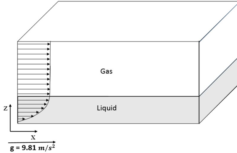
**Fig. 2** Parabolic velocity profile for falling film initialisation.
