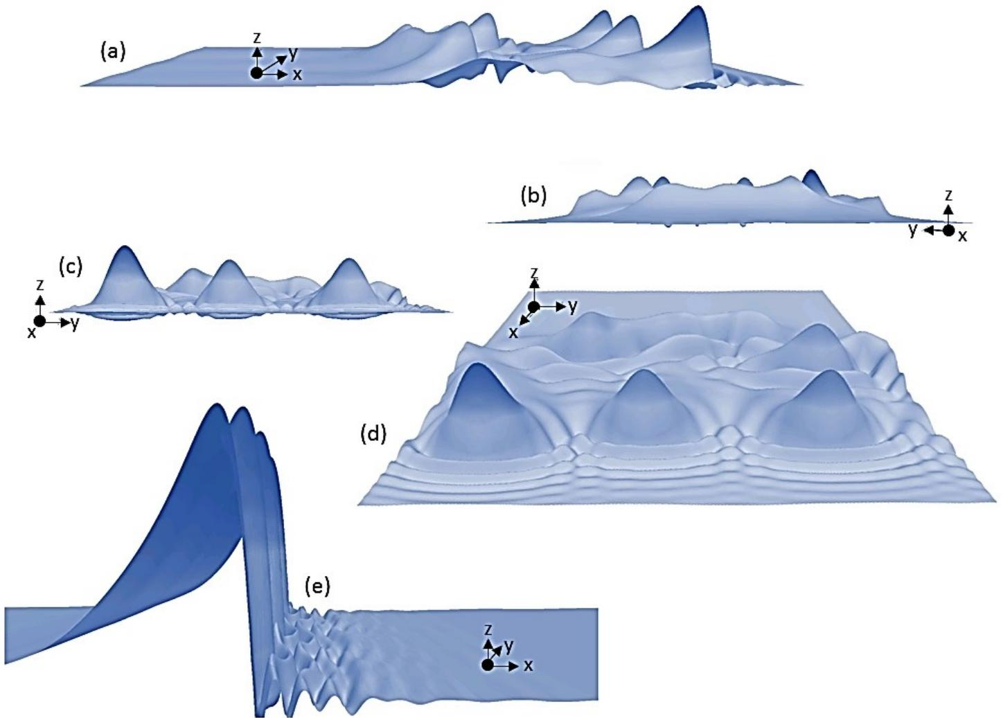
**Fig. 4** Typical interface profile of disordered three-dimensional solitary waves on a flowing liquid film. The simulation parameters are same as in Fig. 5.3. Here, the interface height has been magnified 30 times to clearly reveal minutes details of the wave features.
