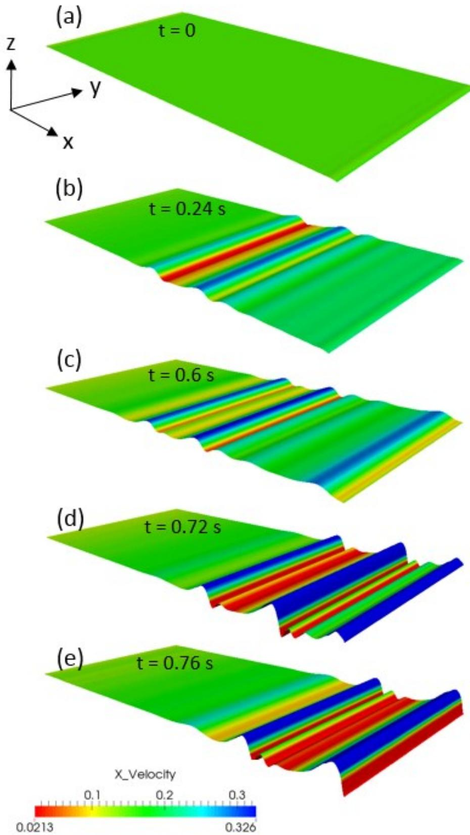
**Fig. 10** Streamwise velocity plot of the gamma II wave family in three dimensions (code Blue). Simulation parameters are  $Re$  62,  $\beta = 90$ ,  $F = 15$  Hz. The interface height has been magnified to clearly reveal the wave propagation. The computed wave speed is 0.233 m/s
