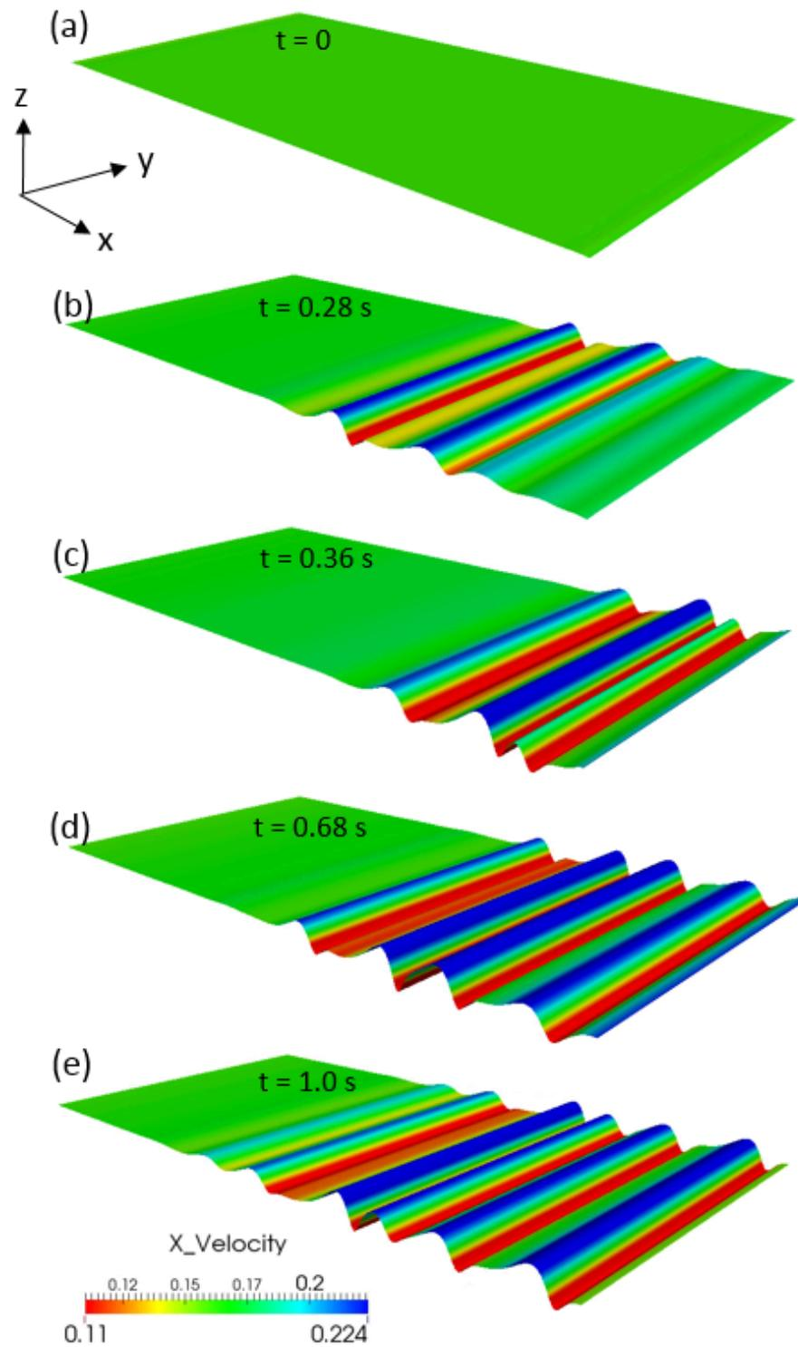
**Fig. 8** Streamwise velocity plot of the gamma I wave family. Simulation parameters are same as in Fig. 5.24. The interface height has been magnified to clearly reveal the wave propagation.
