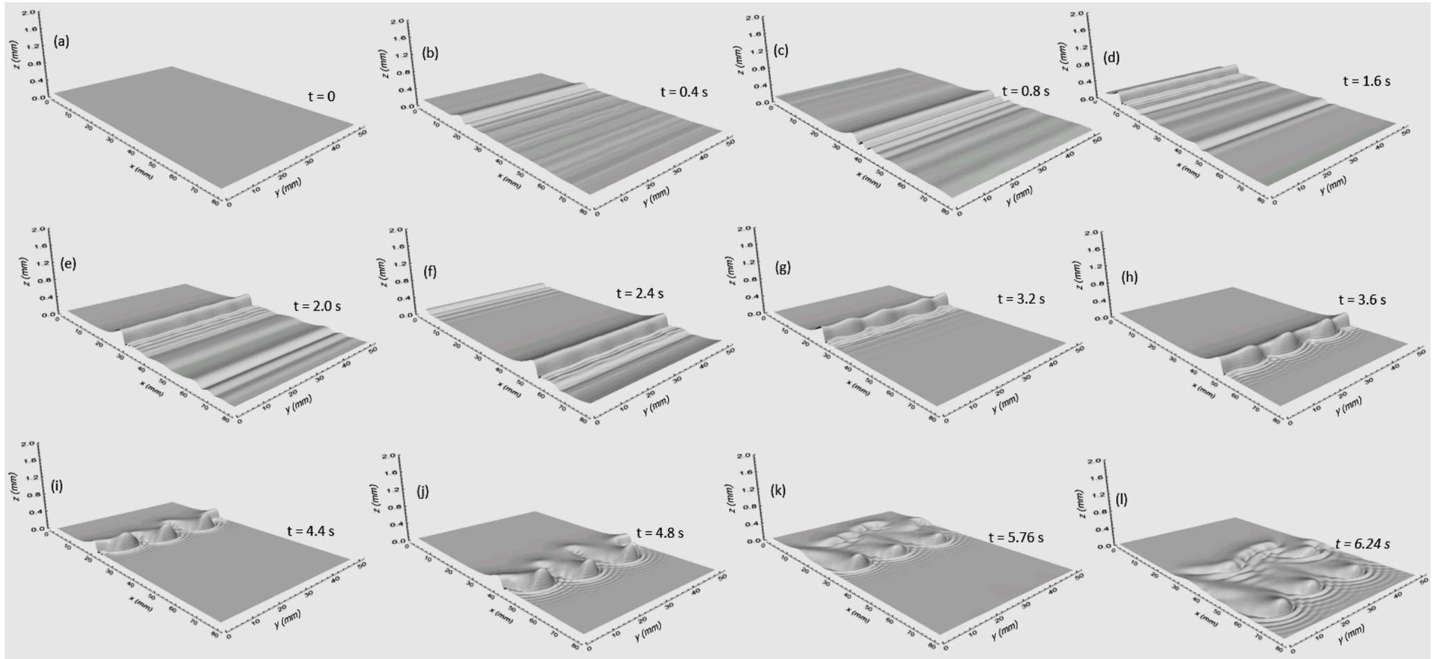
**Fig. 3** Time-propagation of naturally developing waves, in three dimensions. Simulation parameters are  $Re = 100$ ,  $\beta = 90$ . The interface height has been magnified 10 times to clearly reveal the wave propagation.
