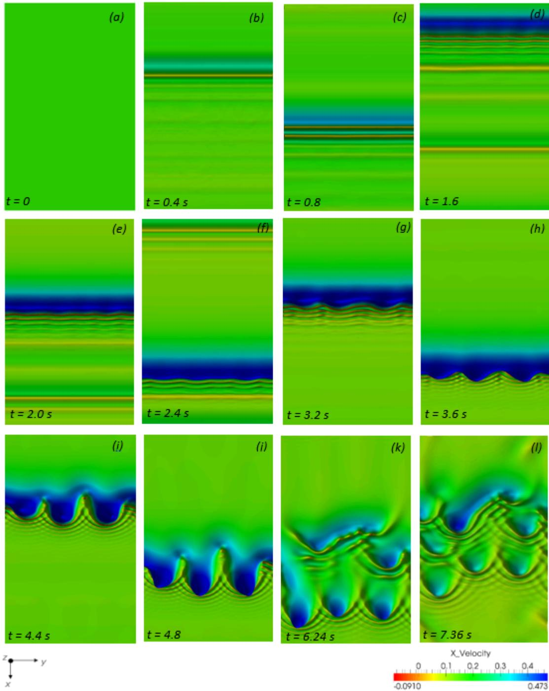
**Fig. 6** Streamwise velocity plot of naturally developing waves, in three dimensions. Simulation parameters are  $Re = 100$ ,  $\beta = 90$ . The interface height has been magnified 10 times to clearly reveal the wave propagation.
