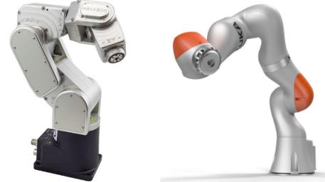
Fig. 1: The KUKA LBR iiwa (right) and the Mecademic Meca500 (left) were examples for collision detection.
