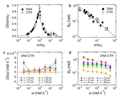
**Figure 3:** (*a*, *b*) Wire average rotation velocity  $\Omega(\omega)$  and oscillation amplitude  $\theta_B(\omega)$  measured in DNA and CTR dispersions. The continuous lines are calculated from the constitutive equations for Newton fluids. (*c*, *d*) Same as 2a and 2b for the 4:1 DNA-CTR complex. For the mixed dispersions,  $\Omega(\omega)$  is close to zero and frequency independent. The oscillation amplitude displays a strong dependency with the wire length.
