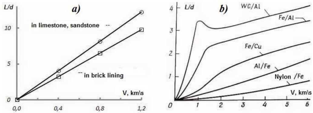
Fig.3. Penetration depths, related to metal balls' diameter, according to the materials [23] of artillery test results (a), penetration depth, related to impactors' diameters, depending on the impact speed for different combinations of projectile and target materials [22] according to the results of laboratory experiments (b).
