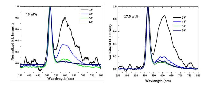
Figure S4: Electroluminescence spectra at various voltages for host/guest PeLEC devices with 10 wt% or 17.5 wt% [Ir(*t*-Bupmtr)<sub>2</sub>(bathophen)][PF<sub>6</sub>] guest.
