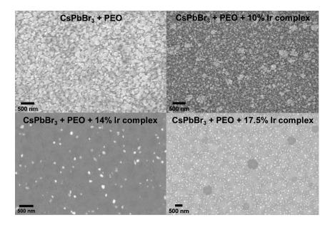
**Fig. 6 Morphology of host-guest films.** Scanning electron microscopy of thin films of CsPbBr<sub>3</sub> + PEO and CsPbBr<sub>3</sub> + PEO + various fractions of [Ir(*t*-Bupmtr)<sub>2</sub>(bathophen)][PF<sub>6</sub>].
