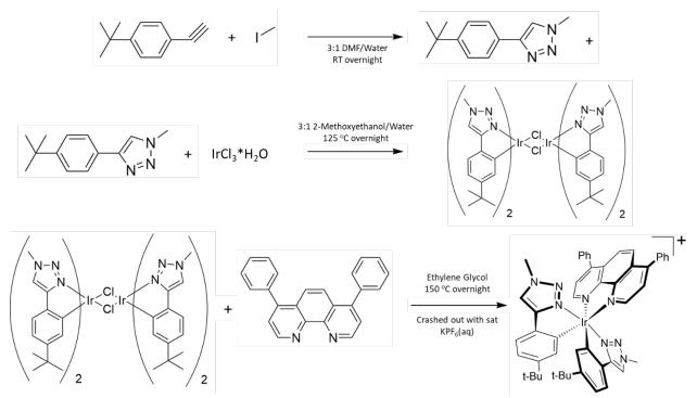
Scheme S1: Synthesis of [Ir(*t*-Bupmtr)<sub>2</sub>(bathophen)][PF<sub>6</sub>]
