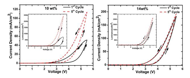
Figure S3: Current density versus voltage for host/guest PeLEC devices with 10 wt% or 14 wt% [Ir(*t*-Bupmtr)<sub>2</sub>(bathophen)][PF<sub>6</sub>] guest.
