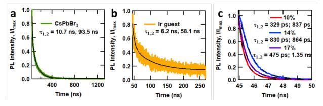
**Fig. 5 Time resolved PL spectroscopy of host, guest, and host-guest films. a** Time resolved PL of a CsPbBr<sub>3</sub> film. **b** Time resolved PL of a [Ir(*t*-Bupmtr)<sub>2</sub>(bathophen)][PF<sub>6</sub>]. **c** Time resolved PL from films of blends of CsPbBr<sub>3</sub> and [Ir(*t*-Bupmtr)<sub>2</sub>(bathophen)][PF<sub>6</sub>] expressed as various weight percentages of [Ir(*t*-Bupmtr)<sub>2</sub>(bathophen)][PF<sub>6</sub>].
