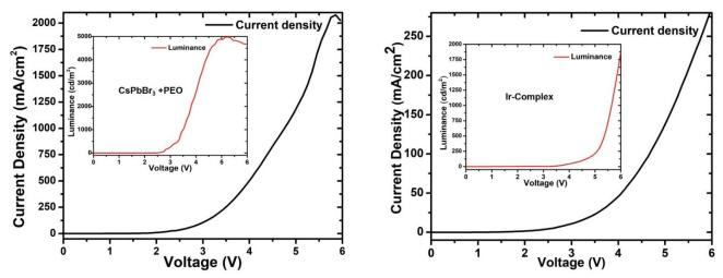
Figure S2: Current density versus voltage and luminance versus voltage (insets) for CsPbBr<sub>3</sub> + PEO and [Ir(*t*-Bupmtr)<sub>2</sub>(bathophen)][PF<sub>6</sub>] (pure guest) PeLECs.
