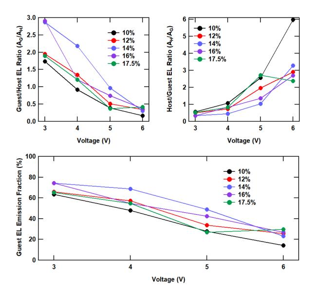
Figure S5: Guest/host and host/guest EL emission area ratios and guest EL emission fraction from the electroluminescence spectra for host-guest PeLECs with various weight fractions of guest at various applied voltages. Peak area ratios were calculated by integrating EL as a function of emission energy for each component peak.
