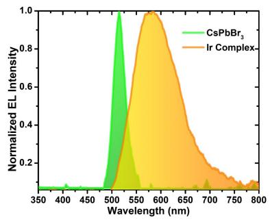
Figure S1: Electroluminescence (EL) spectra at 4.0 V for CsPbBr<sub>3</sub> + PEO (host and electrolyte) and [Ir(*t*-Bupmtr)<sub>2</sub>(bathophen)][PF<sub>6</sub>] (pure guest) PeLECs.
