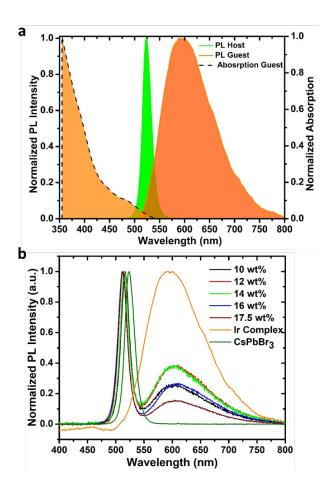
Fig. 1 Thin film photoluminescence (PL) and absorbance spectra. a Normalized PL of thin films of the CsPbBr<sub>3</sub> host and the  $[Ir(t-Bupmtr)_2(bathophen)][PF_6]$  guest, as well as thin film absorbance of the  $[Ir(t-Bupmtr)_2(bathophen)][PF_6]$  guest. b Normalized thin film PL of the CsPbBr<sub>3</sub> host, the  $[Ir(t-Bupmtr)_2(bathophen)][PF_6]$  guest, and host guest blends of various percent by weight guest.
