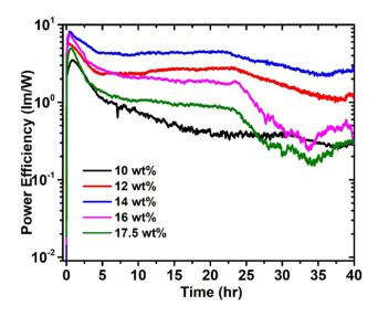
Figure S7: Power efficiency versus time for host/guest PeLEC devices with various weight fractions of guest operating at 1.0 mA constant current.
