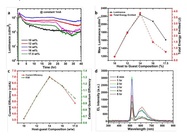
**Fig. 4 PeLEC operation under constant current and constant voltage driving. a** Luminance vs. time for host-guest PeLECs with various weight fractions of guest under 1.0 mA constant current driving (current density 0.33 mA/cm<sup>2</sup>). **b** Maximum luminance and total emitted energy
