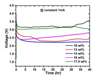
Figure S6: Voltage versus time for host/guest PeLEC devices with various weight fractions of guest operating at 1.0 mA constant current.
