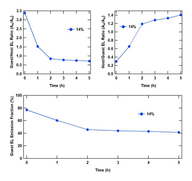
Figure S8: Guest/host and host/guest EL emission area ratios and guest EL emission fraction as a function of time from the electroluminescence spectra for host-guest PeLECs with 14 wt% guest. Peak area ratios were calculated by integrating EL as a function of emission energy for each component peak.
