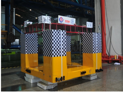
(a) Semi-submersible model (1:60).
