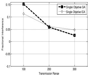
Figure 8. The values of fractional interference for GICA and ICA channel assignment schemes. For a network with a large number of clusters, approx. 30 clusters, ICA has lower fractional interference (see dashed-dotted line for transmission range of 100).
