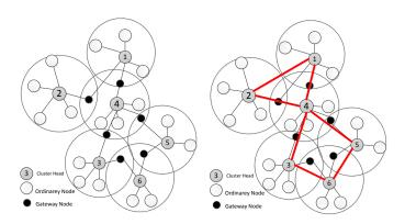
Figure 1. A clustered ad hoc network; the G(V, E) is determined by the graph.
