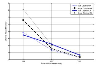
Figure 7. The obtained values of channel reuse efficiency using GICA and GGA. For multi-objective function, the channel reuse efficiency is lower than the single-objective function (blue solid and dotted lines).
