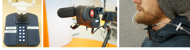
Figure 1: Control interfaces used in this study. From left to right: 3-axis joystick, head array system, sip/puff switch.
