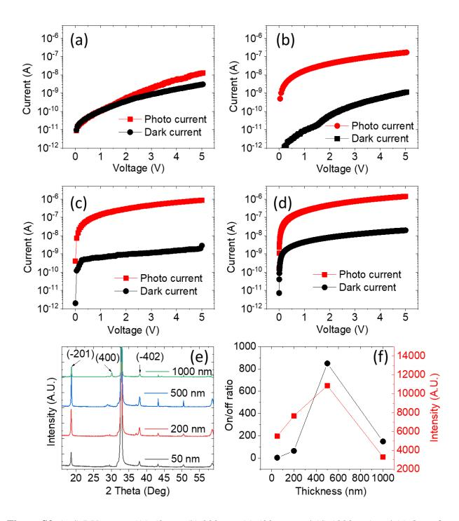
**Figure S3.** (a-d) I-V curves ((a) 50 nm, (b) 200 nm, (c) 500 nm, and (d) 1000 nm) and (e) Out-ofplane theta–2 theta XRD patterns measured on the samples with different  $\beta$ -Ga<sub>2</sub>O<sub>3</sub> thickness. (f) Evolution of the on/off ratio and the intensity of  $\beta$ -Ga<sub>2</sub>O<sub>3</sub> (-201) diffraction peak with film thickness. The results indicate that the sample coated with 500 nm Ga<sub>2</sub>O<sub>3</sub> film has an optimized
