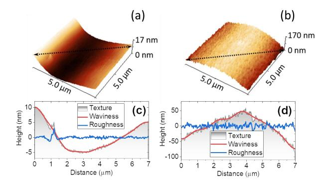
**Figure 4** 3D AFM images (a, b) and height profiles along the black dashed lines (c, d) of the buffered tape and the  $\beta$ -Ga<sub>2</sub>O<sub>3</sub> coated flexible tape, including texture, waviness and roughness.
