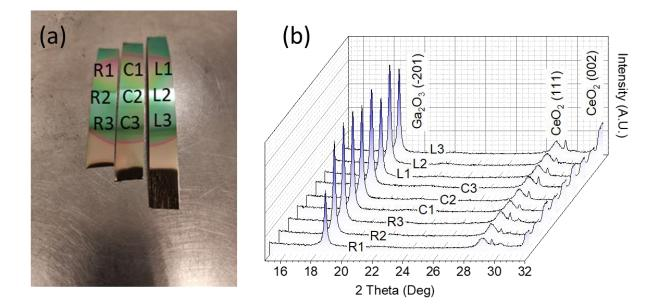
**Figure S4.** (a) Photograph of a batch of samples including three tapes that took out from the PLD chamber after  $\beta$ -Ga<sub>2</sub>O<sub>3</sub> deposition, which is the same as Figure 1(c) except with the position indicators. (b) Out-of-plane 2 theta XRD patterns measured at the various positions marked in (a).
