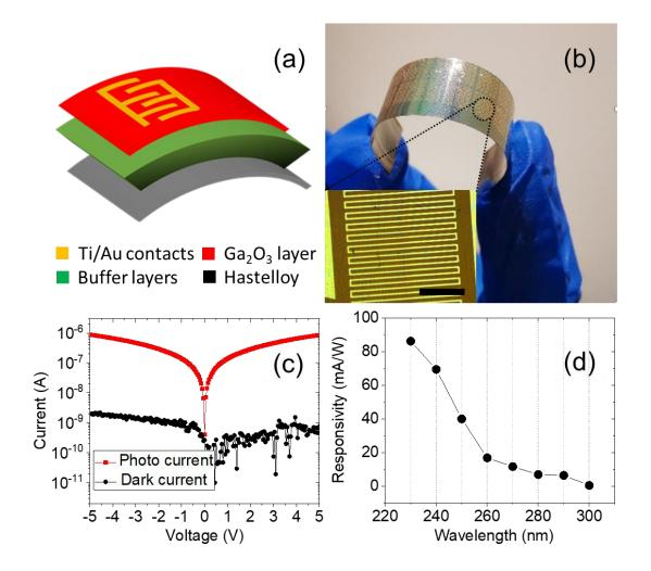
**Figure 5.** (a) Simplified schematic illustration and (b) photograph of the flexible PD based on the  $\beta$ -Ga<sub>2</sub>O<sub>3</sub> coated semiconductor tape, and the inset shows a microscopic photograph of the Ti/Au electrode array with a scale bar equals to 100 µm. (c) I-V characteristics of the sample tested in dark and under 254 nm illumination. (d) Wavelength-dependent responsivity of the sample.
