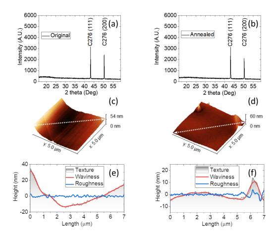
**Figure S1.** (a, b) Out-of-plane 2 theta XRD patterns and (c, d) 3D AFM images of the hastelloy tape before and after annealing at 800 °C for 3 hours. (e, f) Height profiles along the white dashed lines in (c, f), including texture, waviness and roughness. Figure (e) and (f) give root-mean-square (RMS) roughnesses of 0.9 and 1.2 nm, respectively. The results indicate that the hastelloy tape is robust against high temperature conditions at least up to 800 °C, since the high temperature
