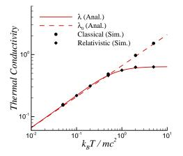
FIG. 5. (color online) Thermal conductivity measured from classical (circles) and relativistic (diamond) molecular dynamics simulations are compared to their corresponding analytical predictions (dashed and solid lines, respectively). Classical as well as relativistic MD show very good agreement with theory in the whole range of temperature parameters. Table I gives more detail.
