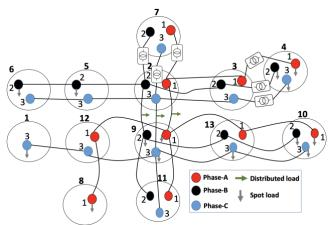
Fig. 2: Phase-connectivity between different nodes of the IEEE 13 node distribution feeder (nodes renumbered in ascending order).
