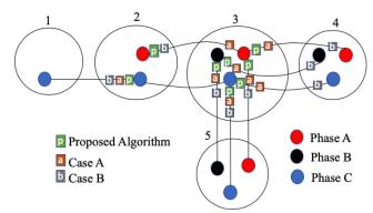
Fig. 3: µPMU placement solutions subject to different objectives.
