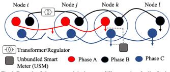
Fig. 1: Example of phase connectivity between different nodes of a distribution network.
