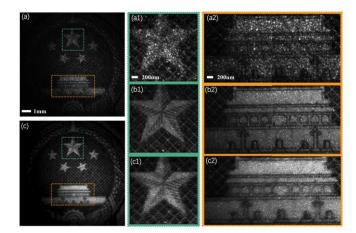
Fig. 3. Reconstructions for the rough object (100 CNY). (a)An entire FOV of raw image captured by our CSAI platform. (c) Image acquired with larger NA, which is almost equivalent to the CSAI synthetic NA of 0.045. (a1, a2) Close-ups of two different sub-regions. (b1, b2) The corresponding reconstructions. (c1, c2) The corresponding regions of ground truth.
