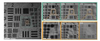
Fig. 2. Performances of the CSAI platform for the smooth object (USAF resolution target). (a) An entire FOV image captured by the CSAI platform. (a1, b1) Enlargement of the raw image. (a2, b2, a3, b3) Intensity and phase reconstructions and their close-ups, respectively, where the feature of group 7, element 2 can be clearly resolved.
