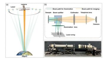
Fig. 1. Schematic and experimental photograph of the CSAI system. (a) The scenario of our CSAI system. (b) Simplified CSAI setup. (c) Photograph of our CSAI system.
