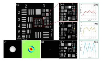
Fig. 4. Indirect verification of the aberrations recovered by our CSAI platform. (a) Entire image captured by the same system with incoherent illumination. (b) Close-up of the central region. (c-e) The amplitude and phase of recovered CTF, and the calculated PSF. (f) Blind deconvolution result. (g) The PSF deconvolution result. (b1-g1) Line profiles of group 5, element 3 in Figs. 4(b-g).
