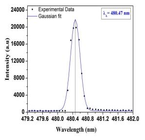
Fig. 3(b) Spectral Line of Ar II in Axial Observation obtained at maximum operating voltage of 15 kV considered as shifted wavelength
