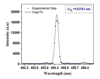
Fig. 4. Voigt fitted profile of 454.50 nm Ar II spectral line
