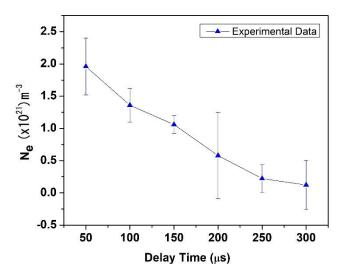
Fig. 7. Plasma density variation as a function of different delay times
