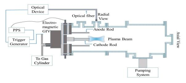
Fig.1. Schematic of Pulsed Plasma Accelerator along with diagnostic arrangement
