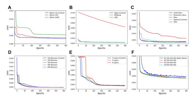
**Figure S2**. Forward dense network hyperparameter tuning. Validation loss of a controlled architecture in comparison to various dependent variables, including: (A) batch size, (B) optimizer, (C) activation function, (D) number of neurons per layer, and (E) number of hidden layers. (F) Final optimized architecture comparison.
