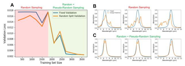
**Figure S6.** Training set size analysis. (A) Validation loss vs. training set size with fixed and randomly split validation datasets. The training set consists of both randomly sampled and pseudo-randomly sampled designs. Test results of a network trained on (B) only randomly sampled designs and (C) both randomly sampled and pseudo-randomly sampled designs.
