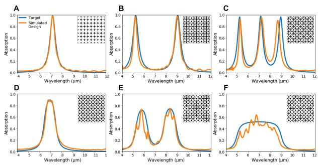
**Figure 3.** Inverse design of new supercell metasurfaces with the tandem neural network. The structures exhibit (A) narrowband, (B) dual-narrowband, (C) triple-narrowband, (D) broadband, (E) dual-broadband, and (F) graybody behaviors. Blue lines indicate the target spectra used as inputs to the network, and orange lines represent the simulated results of the output design parameters. Inset images show the physical layouts of the network-generated supercells.
