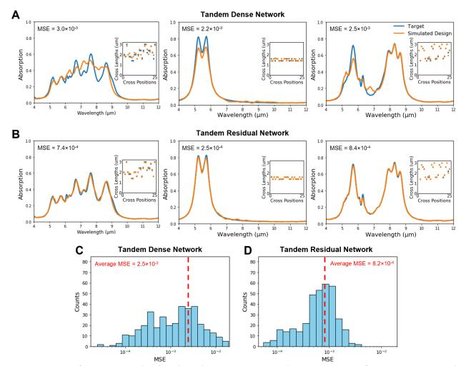
**Figure 2.** Performance evaluation based on mean-squared error (MSE) of target spectra and simulated designs for (A) the tandem dense and (B) tandem residual networks. The tandem residual network achieves a lower MSE for three distinct targets. Inset images show the design parameters for the corresponding spectra. Statistical analyses across the entire validation dataset (over 300 spectra) for the tandem dense (C) and residual (D) networks indicate that the latter achieves a lower average MSE.
