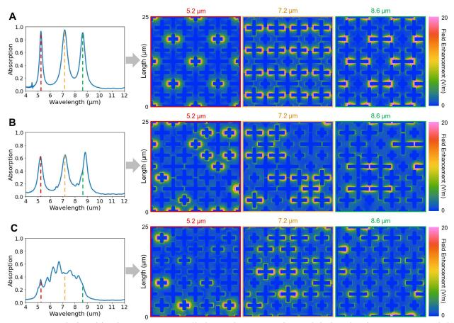
**Figure 4.** Relationships between supercell absorption properties and their subunit resonator spatial distributions. Simulated absorption spectra (of the tandem network-designed structures) and corresponding electric field profiles are shown for triple-narrowband structures with (A) high and (B) low absorption peaks and a (C) graybody structure. These plots reveal the dependence of absorption response on resonator geometry and position relative to other elements.
