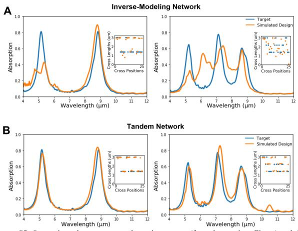
**Figure S5.** Comparisons between target absorption spectra (from the previous Figure) and the simulated spectra for the optimized designs from the (A) inverse-modeling network and the (B) tandem network. The tandem network has greater accuracy in predicting design parameters than the inverse network due to stronger convergence. Inset images show design parameters for the corresponding spectra.
