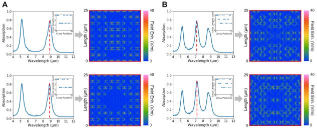
**Figure S4.** Examples of nonuniqueness in the training dataset. Two very different supercell design layouts have nearly-identical (A) dual-band and (B) triple-band absorption responses. Inset images show the design parameters corresponding to the shown absorption spectra.
