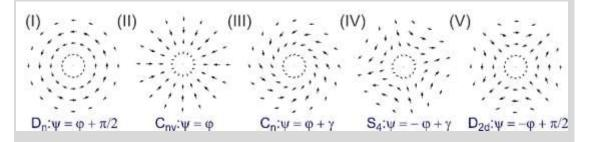
In-plane projections of the magnetization vector in this figure describe *five* different skyrmion core configurations [1-4]. In ferromagnets with  $C_n$  and  $S_4$  symmetries,  $\gamma$  is a constant phase angle determined by the ratio of competing Dzyaloshinskii-Moriya interactions along orthogonal axes [1, 4]. For all five types of skyrmions, the equilibrium profiles  $\theta(\rho)$  are derived from equation
