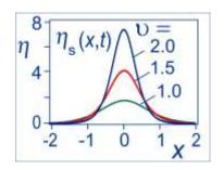
In extremely shallow water when h is a factor 20 or more smaller than the wavelength L, the last term suppresses dispersion processes and stabilizes solutions for solitary waves with bell-shaped profiles (*solitons*) [21]
