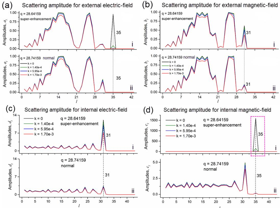
Figure 5. Scattering amplitudes for factors of  $a_l$ ,  $b_l$ ,  $c_l$ , and  $d_l$  against order mode  $-l$  for the spheres with  $q = 28.64159$  and  $q = 28.74159$  on 4 loss levels
