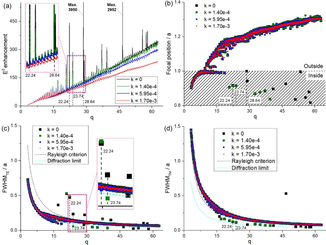
Figure 1. (a)  $|E^2|$  peak field enhancements, (b) normalised focal lengths, (c) and (d)  $FWHM_{TE}$  and  $FWHM_{TM}$ , in the function of  $q$  with  $k = 0, 1.4e-4, 5.95e-4,$  and  $1.70e-3$ .
