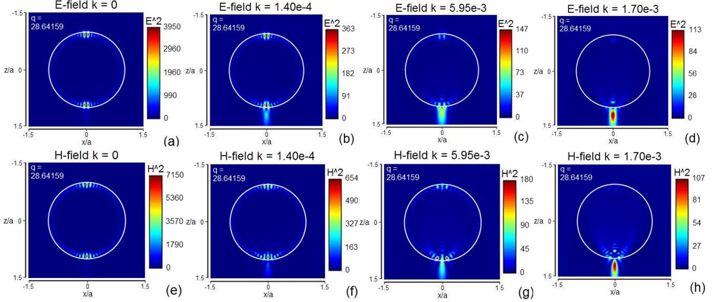
Figure 3. Distributions of  $|E^2|$  (a-d) and  $|H^2|$  (e-h) field intensities for the sphere with  $q = 28.64159$  at the loss levels of  $k = 0, 1.40e-4, 5.95e-4,$  and  $1.70e-3$  in TM mode.
