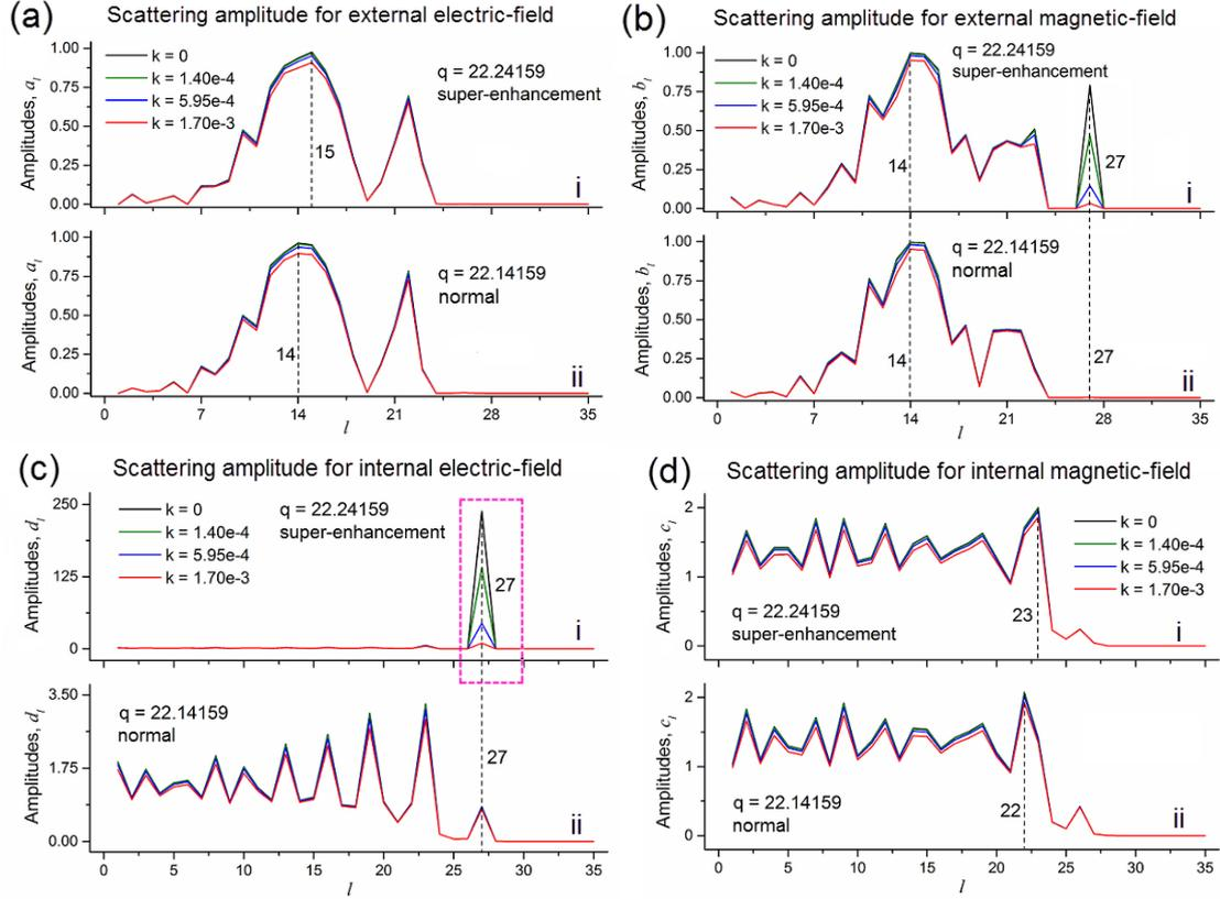
Figure 4. Scattering amplitudes for factors of  $a_l$ ,  $b_l$ ,  $c_l$ , and  $d_l$  against order mode  $-l$  for the spheres with  $q = 22.24159$  and  $q = 22.14159$  on 4 loss levels
