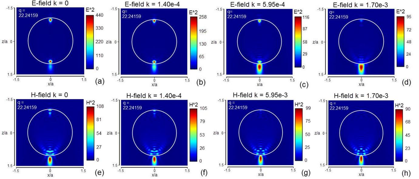
Figure 2. Distributions of  $|E^2|$  (a-d) and  $|H^2|$  (e-h) field intensities for the sphere with  $q = 22.24159$  at the loss levels of  $k = 0, 1.40e-4, 5.95e-4,$  and  $1.70e-3$  in TM mode.
