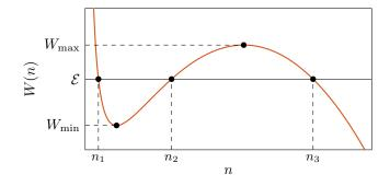
FIG. 1. Schematic behavior of the potential W as a function of n. The value of W at the local minimum (maximum) is  $W_{\min}$  ( $W_{\max}$ ).  $n_1 \leq n_2 \leq n_3$  are the roots of  $W(n) = \mathcal{E}$ .
