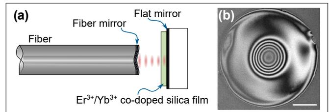
**Fig. 1.** Schematic of the FFPC for lasing. (a) The FFPC is formed by a concave fiber mirror and a flat mirror. An  $\text{Er}^{3+}/\text{Yb}^{3+}$  co-doped silica film (thickness of  $35.1 \mu\text{m}$ ) is set inside the cavity, and bonded onto the flat mirror. (b) An interferometric image of the concave surface of the fiber mirror (with the scale bar of  $30 \mu\text{m}$ ), the radius of curvature of the concave mirror is calculated as  $100 \mu\text{m}$  from the concentric fringes.
