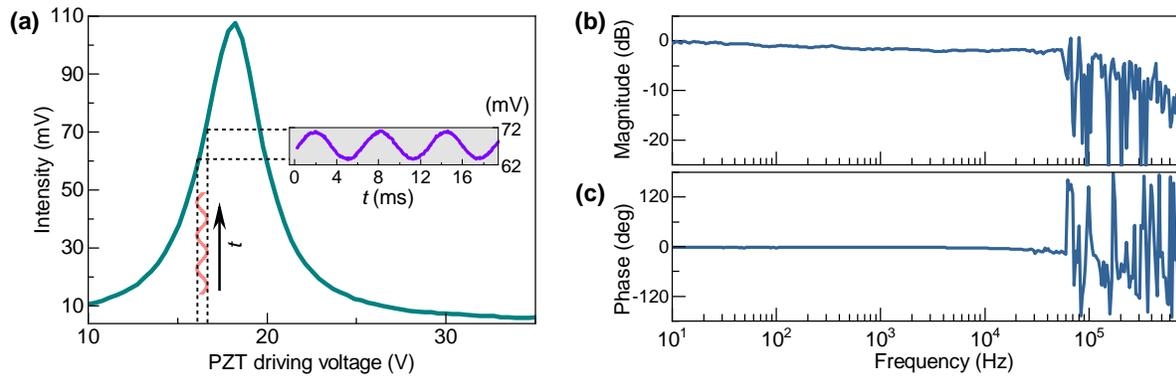
**Fig. 5.** Mechanical bandwidth of the laser device by measuring the driving response. (a) The envelope of the transmission spectrum in green and the spectrum response driven by the small sinusoidal signal. (b) Frequency response diagram of the assembled laser device. From both magnitude and phase variations, the first direct resonance is indicated at 60 kHz.
