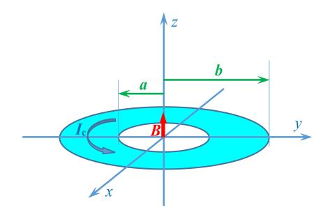
Figure 1. Schematic diagram of the model. The vector of magnetic flux density in the center of the disk, *B*, is shown.
