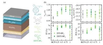
Figure 1. (a) Photovoltaic device structure with chemical structures of the materials used as extraction layers (b) Photovoltaic performance parameters of devices with increasing HBL thickness and reference BCP devices. Concentration ranges from 0.25 mg/ml to 1 mg/ml in methanol.
