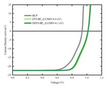
Figure 5. Simulated J-V curves of reference BCP hole-blocking layer and the two dipoles with different LUMO energies.
