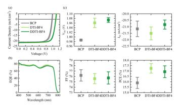
Figure 4. a) J-V-curves for champion devices with each HBL measured under one sun illumination d) External quantum efficiency spectra for each type of device. (c) Photovoltaic parameters statistics of 30 photovoltaic devices.
