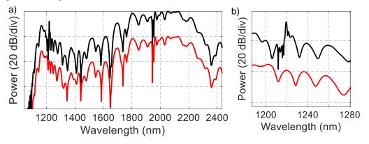
Fig.4 a). Simulated supercontinuum with (black) and without grating (red) with waveguide parameters similar to Fig.2. b) Zoomed-in spectra near the grating response. Plots are shifted vertically for clarity.
