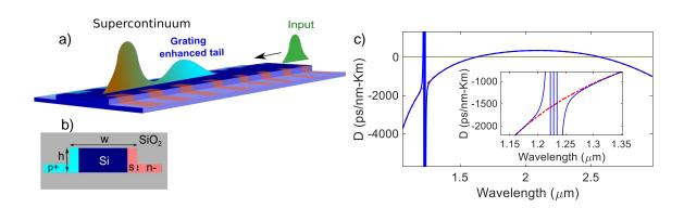
Fig.1 a) The schematic of the device with the input and the output pulse. b) The crossection of the waveguide and c) the dispersion of the waveguide with (solid blue) and without grating (red dash), zoomed in near the Bragg resonance (inset).
