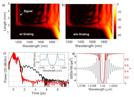
Fig. 5 a) and b) The spectrogram of the supercontinuum evolution with and without grating, respectively. c) The temporal profile of the pulse with (black) and without grating (red) at the output. A tail of the enhanced signal is seen spanning from 2 to 5 ps (black). The group delay (GD) for the grating is shown in the inset. d) The grating transmission (red) and the group delay dispersion (black dash).
