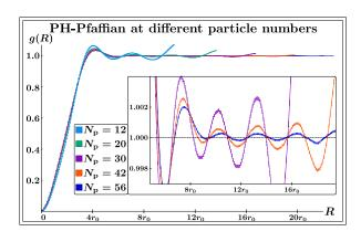
Figure 7. The density-density correlation function of the PH-Pfaffian trial state shows a global suppression of the  $2k_{\rm F}$  amplitudes with increasing particle number, but almost no change in the *R* dependence.
