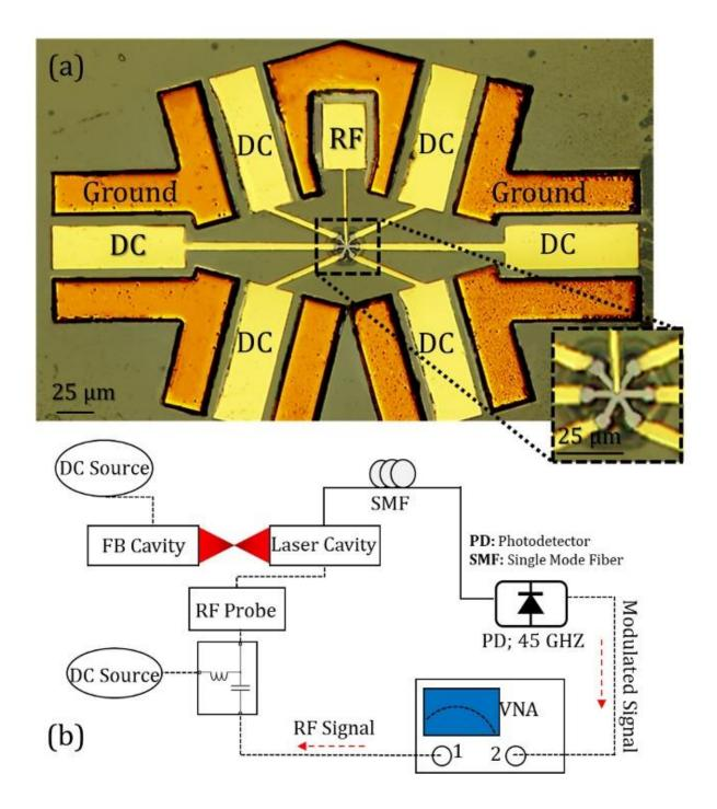
**Figure 3.** (a) The top-view false optical microscopic image of the fabricated MTCC VCSEL with aperture size of  $3.5 \times 3.5 \ \mu m^2$  for inner cavity and six identical feedback, each with a length of 12  $\mu m$ . With an aim to achieve high power, single-mode operation, the Vernier effect in lateral integration in a VCSEL can be utilized to form a larger aperture size and hence, more gain medium <sup>[25,26]</sup>, and (b) our calibrated 45 GHz small signal measurement setup.
