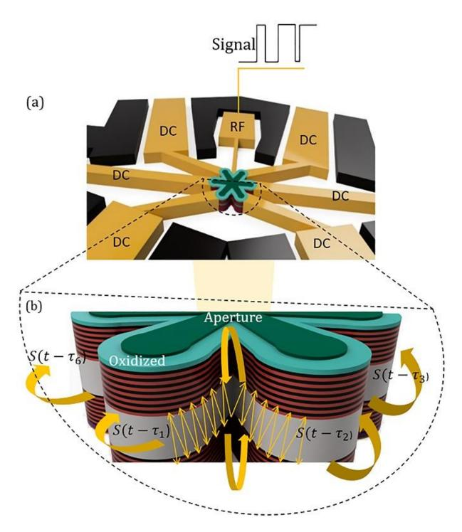
**Figure 1.** Schematic structure of our hexagonal transverse coupled cavity VCSEL (a) Top view, and (b) Cross section view. The six outer cavities are designed to have the same resonant wavelength  $\omega$  at  $I_{feedback} < I_{th}$ .  $I_{laser} = mI_{th}$ . When  $I_{laser}$  increases resonant wavelength red shift like its conventional VCSEL.
