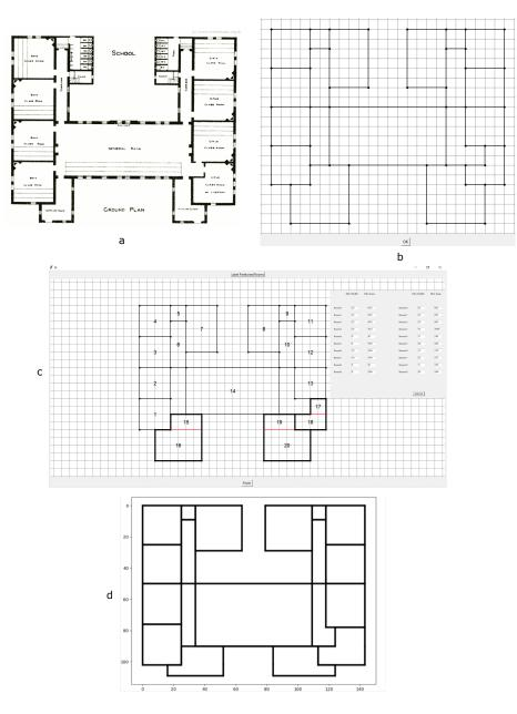
**Fig. 27.** a) Banstead Home School Plan by Higginbotham [49] b) Drawing the Banstead Home School Plan on a GUI generated by GPLAN c) Partitioning of rectilinear rooms and dimensional constraints d) Re-generated Banstead Home School Plan (with new dimensions) by GPLAN
