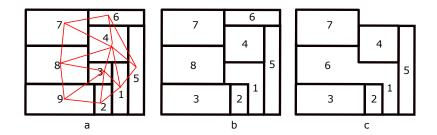
**Fig. 2.** Floorplans Typology a) Rectangular floorplan (RFP) b) Orthogonal floorplan (OFP) c) Irregular floorplan (IFP)
