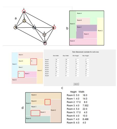
Fig. 24. a) A PTG which is not a PTPG b) Dimensionless OFP generated by GPLAN corresponding to given PTG c) Partitioned OFP and dimensional constraints d) Dimensioned OFP generated by GPLAN
