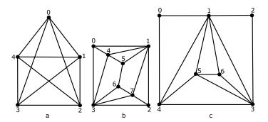
**Fig. 4.** Graphs that are not PTPGs a) A non-planar graph b) A non-triangulated graph c) A PTG with a separating triangle ( $\triangle 153$ )
