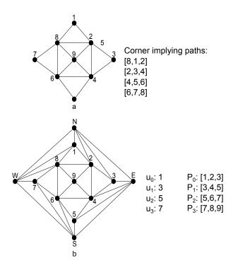
Fig. 13. a) A PTG with corner implying paths b) A PTPG derived from given PTG by using 4-completion considering  $u_i(i = 0, 1, 2, 3)$  as corner vertices
