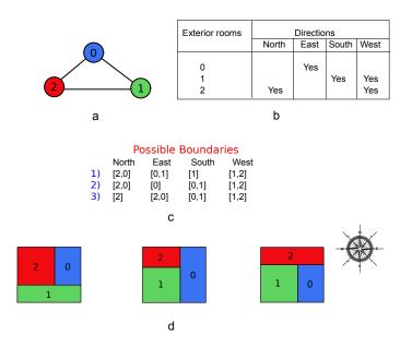
Fig.28. a) An adjacency graph b) User-defined constraints c) Possible boundaries based on user-defined constraints d) Floor plans restricted to user-defined boundary constraints
