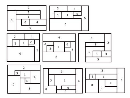
Fig. 22. Out of 256 solutions, which can be obtained using GPLAN, a few OFPs corresponding to the input graph in Figure 17b
