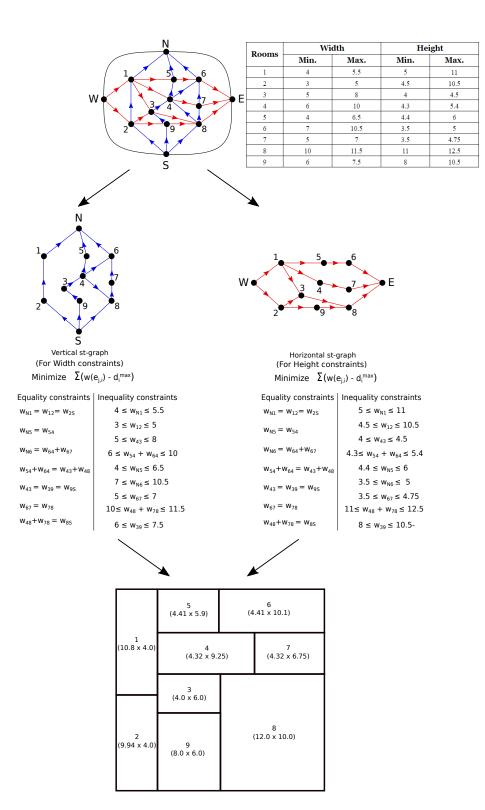
Fig. 23. Dimensioning model based on network flow and linear optimization
