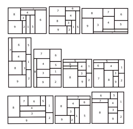
Fig. 21. Out of 1300 solutions, which can be obtained using GPLAN, a few RFPs corresponding to the input graph in Figure 15
