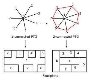
Fig. 10. 1-connected and bi-connected PTGs and corresponding floorplans
