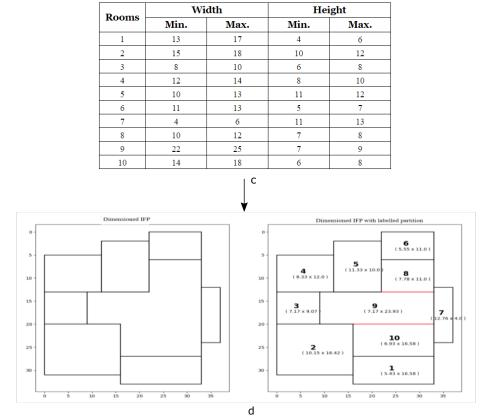
**Fig. 25.** Construction of a dimensioned irregular floorplan a) Dimensionless IFP as input b) IFP transformed into a RFP by adding extra rooms (red) and partitioning orthogonal rooms into rectangles (yellow) c) Dimensional requirements d) Resulting dimensioned IFP obtained using GPLAN
