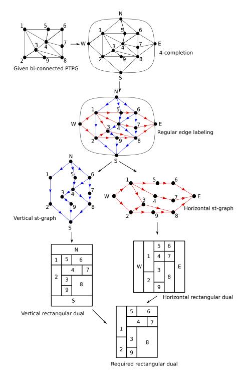
Fig. 15. Construction of a RFP corresponding to a given bi-connected PTPG
