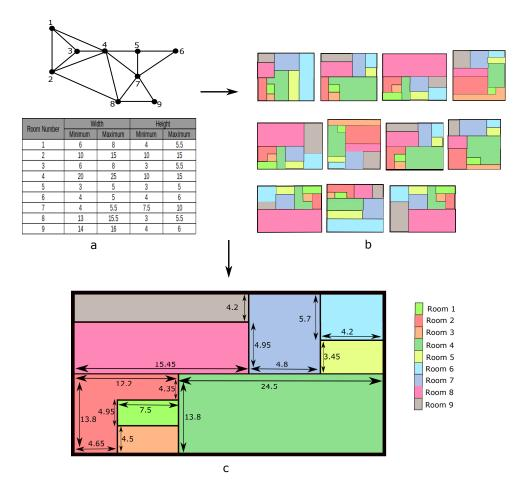
Fig. 1. The working of GPLAN: Illustrating the input format of GPLAN and output produced by it a) Input adjacency graph and dimensional constraints b) Multiple dimensionless floorplans satisfying all the adjacency requirements c) A dimensioned floorplan obtained from the dimensionless floorplans satisfying all given dimensional constraints
