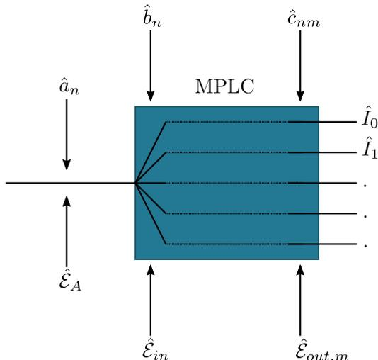
FIG. 6. We introduce in this figure the different notations used to describe the successive steps of the demultiplexing process. The complex field operators are denoted as  $\hat{\mathcal{E}}$  and their associated annihilation operators as  $\hat{a}, \hat{b}, \dots$ . The intensity operators at the outputs of the demultiplexor are written as  $\hat{I}$ .
