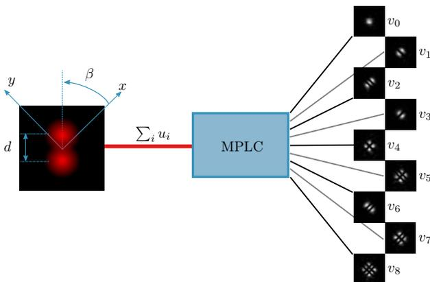
FIG. 2. The beams which enters the MPLC system can be described as a superposition of modes  $u_{0 \leq i \leq 8}$ . Each input mode is demultiplexed and sent to a spatially separated spatial mode  $v_{0 \leq i \leq 8}$ . Each of these modes is coupled into a separate single-mode fiber.
