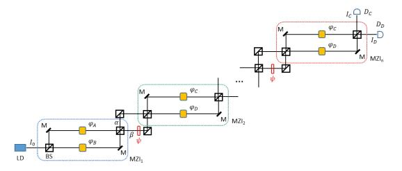
**Figure 1.** An n-folded MZI system. Each  $\varphi_j$  has two bases,  $\varphi_j \in \{0, \pi\}$ . The phase  $\psi$  satisfies  $\psi \in \{0, \pi\}$ . LD, laser diode; I, isolator; C, optical cavity; M, mirror; BS, beam splitter;  $\varphi_j$ , phase in each path; induced by path-length or frequency difference;  $\psi$ , control phase; D, detector;  $I_0$ , input field intensity.
