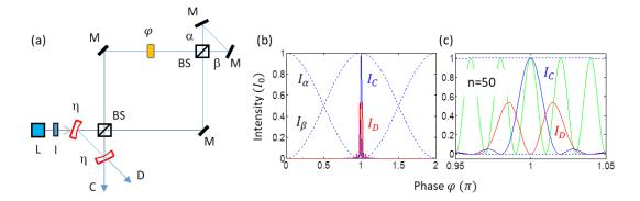
**Figure 3.** Cavity CBW. (a) Schematic of cavity CBW. (b) and (c) Numerical calculations for (a). LD, laser diode; I, isolator;  $\eta$ , Reflection coefficient of an optical cavity; M, mirror; BS, beam splitter;  $\alpha/\beta$ : optical fields; n=number of ACD-MZI in Fig. 1.  $I_{\alpha}/I_{\beta}$ : output intensity of MZI<sub>1</sub>. Green curve in (c):  $I_{c}$  from Fig. 1 for n=50.
