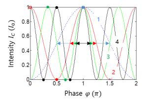
**Figure 2.** Numerical calculations for the output intensity of ACD-MZI of Fig. 1. q=1 (dotte), q=1 (red), q=3 (green), and q=4 (black). For simplicity  $\varphi_B = \varphi_D = 0$  is set for  $\varphi_C = -\varphi_A$  to satisfy the asymmetry coupling in CBW with  $\psi = 0$  [28].  $I_C$  equivalent to  $(I_A)^n$  in the n-coupled MZI in Fig. 1. The colored arrows indicate each full width at half maximum.
