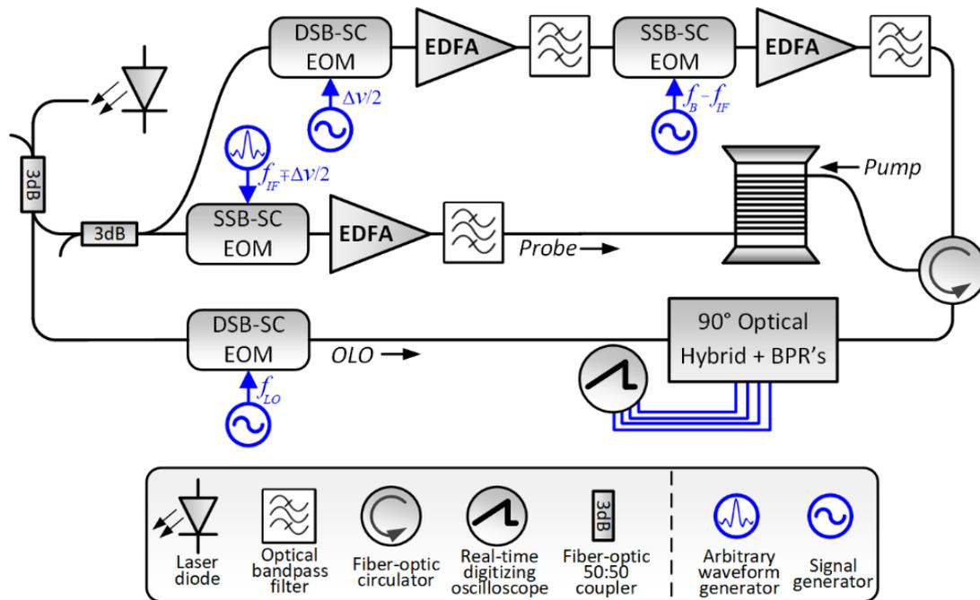
Figure 6: **Simplified schematic illustration of the experimental setup.** S/DSB-SC EOM: single/double-sideband suppressed-carrier electro-optic modulator; EDFA: erbium-doped fibre amplifier; BPR: balanced photo-receiver; OLO: optical local oscillator.
