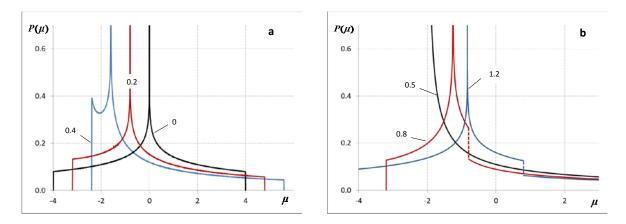
Fig. 3. Spectral density  $P(\mu)$  for 2D Ising system and different values of constant of interaction with next nearest neighbors. (a) When  $0 \le b < 0.5$ , b = 0, 0.2, and 0.4; (b) When  $b \ge 0.5$ , b = 0.5, 0.8, and 1.2. Dotted lines define jumps of spectral density.
