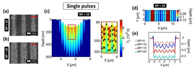
FIG. 5 Surface pattern upon *single* pulse irradiation with  $\Lambda_{DLIP} \sim 5500$  nm. SEM images of stainless steel surface for NP=10 (a) and NP=50 (b). (c) Modelling of the temperature profile and the flow vectors 450 ps after NP = 9. (d) Calculated surface profile after NP = 10. (e) Depth profile along *white* dashed line in (d) for NP=5, 10, 15, 20. *Red* double-ended arrow in (a) and (b) indicates polarization direction.
