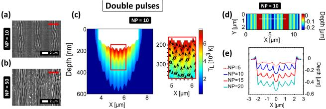
FIG. 6 Surface pattern upon *double* pulse irradiation with  $A_{DLIP} \sim 5500$  nm. SEM images of stainless steel surface for NP=10 (a) and NP=50 (b). (c) Modelling of the temperature profile and the flow vectors 505 ps after NP = 9. (d) Calculated surface profile after NP = 10. (e) Depth profile along *white* dashed line in (d) for NP=5, 10, 15, 20. *Red* double-ended arrow in (a) and (b) indicates polarization direction.
