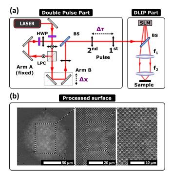
FIG. 1. (a) Experimental setup of combined DLIP and DP. Abbreviations: Half-waveplate (HWP), Linear polarizing cube (LPC), Beamspliter (BS), Spatial Light Modulator (SLM), focusing lens (f) (b) Surface processed with 4 beams with  $\theta_n = 19 \pm 0.5$ °, NP = 50 and 42 µJ per pulse.
