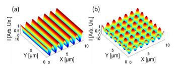
FIG. 2. Normalised intensity distribution for (a) two- and (b) fourbeam interference. Periodicities equal to P=1650 nm along *x*-axis (for (a)) and *x*- and *y*-axis (for (b)) have been selected.
