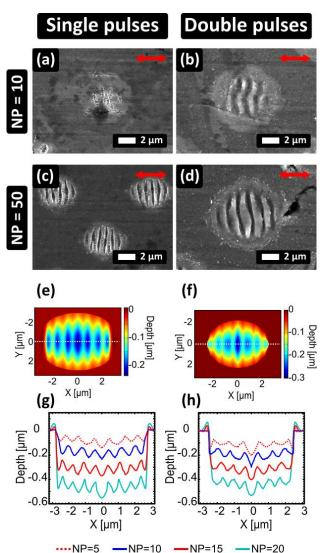
FIG. 8 SEM images of stainless steel surface *irradiated* with  $\Lambda_{DLIP}$  ~7600 nm with single (a,c) and double pulses (b,d) with NP = 10 and 50, respectively. Simulation results of the surface profile obtained with NP = 10 are shown for SP (e) and DP (f). Depth profile along *white* dashed lines in (e) and (f) for NP=5, 10, 15, 20 are shown in (g) and (h).
