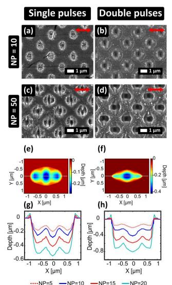
FIG. 7 SEM images of stainless steel surface irradiated with  $A_{DLIP} \sim 2262$  nm with single (a,c) and double pulses (b,d) with NP = 10 and 50, respectively. Simulation results of the surface profile obtained with NP = 10 are shown for SP (e) and DP. Depth profile along *white* dashed lines in (e) and (f) for NP=5, 10, 15, 20 are shown in (g) and (h).
