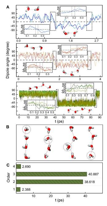
**Fig. 2.** The snapshots of trajectories for the typical molecular orientation of water chains. (A) The change of dipole angle for each water molecule in the different chain. Here, different color indicates different number of water molecules. (B) The flip process of water tetramer chain. (C) Comparison of the rotation time of each water molecule for the tetramer chain.
