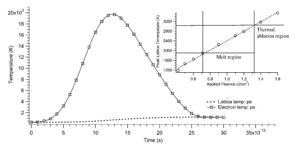
Figure 8 Electron and lattice temperatures after onset of laser irradiation with a 10 ps 1030 nm pulse, with an applied fluence of 1.9 Jcm<sup>2</sup>. The peak lattice temperature is 4000 K Inset: Change in peak lattice temperature with applied fluence, from 0.42- 1.6 Jcm<sup>2</sup>
