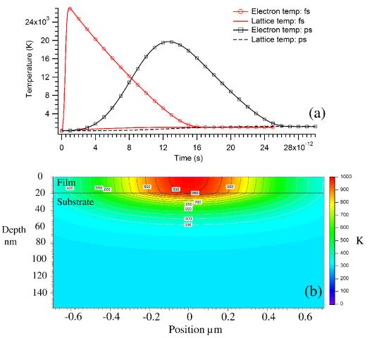
Figure 5 (a) Peak electron and lattice temperature after laser irradiation with fs and ps pulses, at their respective threshold fluences (b) Peak temperature in the film and substrate, 20 ps after irradiation with a 0.32 Jcm<sup>-2</sup> fs pulse.
