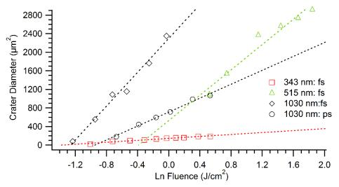
Figure 2: Fluence dependence of the crater diameter squared for ps and fs pulses, at wavelengths of 343, 515 and 1030 nm.
