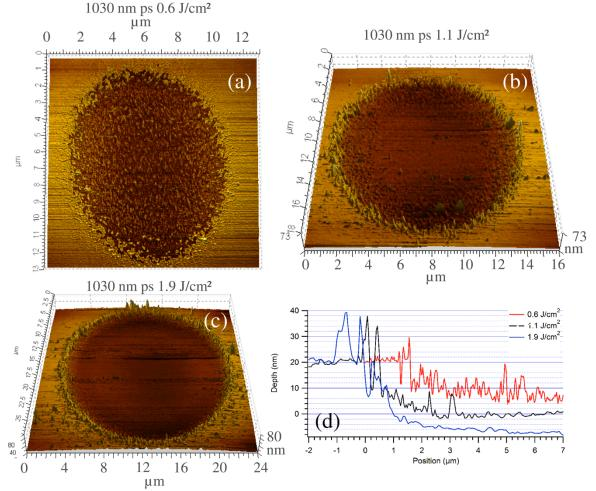
Figure 5: ITO on glass craters after ps laser irradiation with applied fluences of (a)  $0.6 \text{ Jcm}^{-2}$  (b)  $1.1 \text{ Jcm}^{-2}$  and(c)  $1.9 \text{ Jcm}^{-2}$  (d) Cross sectional craters profile at applied fluences of 0.6, 1.1 and  $1.9 \text{ Jcm}^{-2}$
