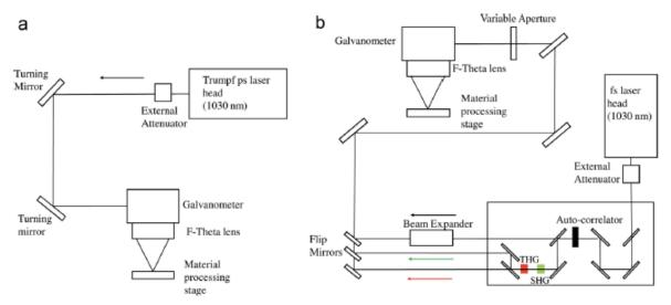
Figure 1 Schematic diagram of the experimental configuration for femtosecond and picosecond pulse durations..
