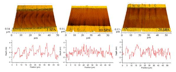
Figure 4 Femtosecond ITO on glass craters at 3, 10, 20 shot per area, at an applied fluence of 1.2 Jcm<sup>-2</sup>. Line profiles present indications of surface topographies in centre along the direction of the scribe.
