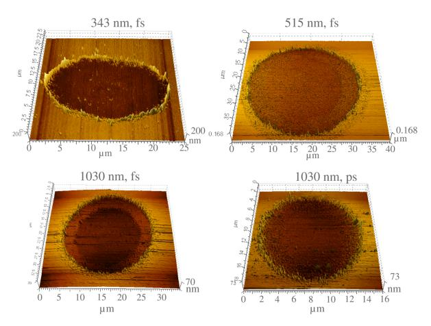
Figure 3 AFM surface topography of ITO on glass craters, showing selective removal of the ITO film, at wavelength of 343 (0.8 J/cm<sup>2</sup>, fs), 515 nm, (1.4 J/cm<sup>2</sup>, fs), 1030 nm (1.2 J/cm<sup>2</sup>, fs) and 1030 nm (1.1 J/cm<sup>2</sup>, ps).
