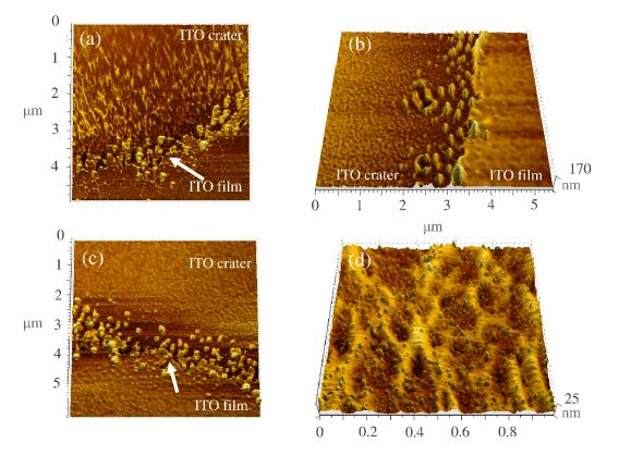
Figure 4 Crater edges for ITO on glass when ablated using (a) 1030 nm ps pulses, (b) 343 nm fs pulses (c) 1030 nm fs pulses. Large particles at the edge are visible at all wavelengths, including evidence of edge cracking at IR wavelengths (See arrows). Re-deposited nanoparticles on in center of crater floor (d) after 1030 nm ps pulses.
