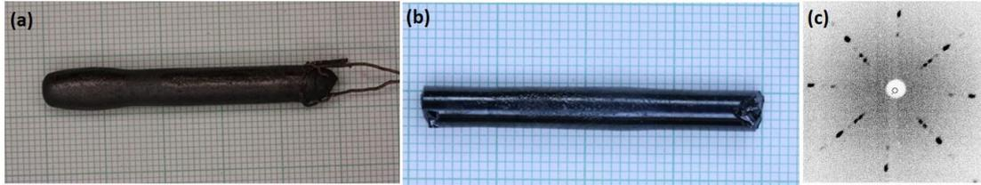
**Figure 8** Photographs of the Nd-LSCO ( $x = 0.19$ ) samples: (a) the ceramic rod used for the crystal growth, (b) the as-grown single crystal from the OFZ furnace growth, (c) Laue diffraction pattern performed on surface of the as-grown single crystal, along the growth direction, [001]. The black spots mark the intensity from the backscattered Bragg peaks, while the white circle shows the centre of the beam.
