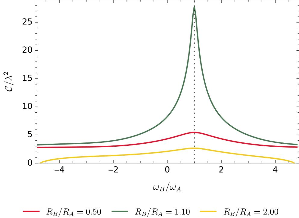
FIG. 10: The concurrence  $\mathcal{C}(\rho_{AB})/\lambda^2$  is plotted as a function of  $\omega_B/\omega_A$  for two detectors concentrically rotating in  $xy$  plane. Here we have set  $\Delta d = 0$ ,  $\omega_A\sigma = 1.00$ ,  $R_A/\sigma = 0.10$  and  $\Omega\sigma = 0.10$ . The vertical dotted line denotes the point  $\omega_B/\omega_A = 1$  at which  $\mathcal{C}(\rho_{AB})/\lambda^2$  will take the maximum value.
