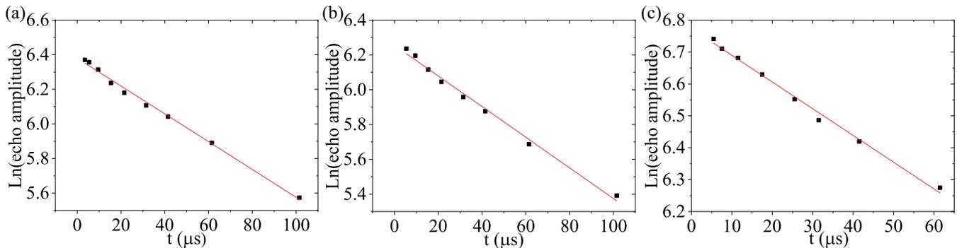
FIG. 2. (color online) Two-pulse photon echo measurements implemented in three different regions inside the sample where  $t$  is the spacing between the two incident pulses. The red solid lines are the results of the linear fitting. (a) In the type-IV waveguide, the coherence time  $T_2$  is fitted as  $124 \pm 4 \mu\text{s}$ . (b) In the bulk-1 area,  $T_2$  is fitted as  $113 \pm 3 \mu\text{s}$ . (c) In the bulk-2 area,  $T_2$  is fitted as  $119 \pm 4 \mu\text{s}$ .
