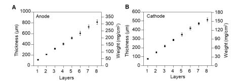
**Supplementary Figure 3**. Thickness calibration of the (A) anode and (B) cathode printed using their corresponding stencils. 5 samples were taken to generate the average thicknesses and standard deviations of each data point.
