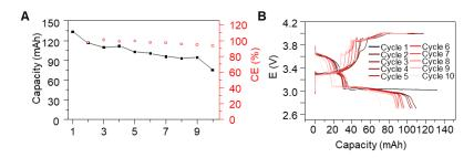
**Supplementary Figure 15**. The cycling of two 8-layer  $2 \times 2$  cm<sup>2</sup> battery connected in series at the rate of 0.05 C.
