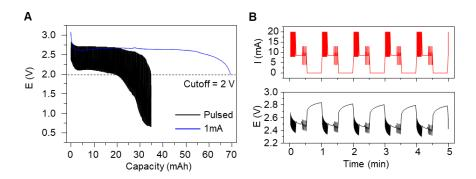
**Supplementary Figure 24**. (A) The discharge curve of a CR1620 Lithium coin cell battery rated at 68 mAh nominal capacity under continuous 1 mA discharge and pulsed discharge. Significant capacity fade is observed for the battery with pulsed discharge. (B) Zoomed in view of the current and voltage change of the CR1620 battery.
