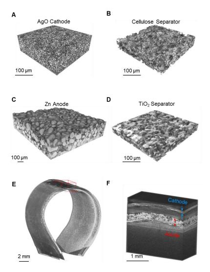
**Supplementary Figure 21**. Additional microscopic 3D images of the (A) cathode, (B) cellulose separator, (C) anode, and (D)  $\text{TiO}_2$  separator generated using the micro-CT. (E) the 3D image of the bent  $1 \times 5 \text{ cm}^2$  battery in a different angle and (F) the zoomed-in view of the top of the cell showing no cracking nor delamination between the layers.
