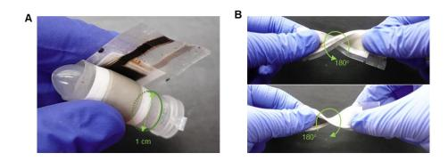
**Supplementary Figure 19**. Additional images illustrating the manual bending and twisting of the battery. (A) A tube with diameter of 1 cm was used to bend the battery for half and one entire round. (B) The battery was twisted counterclockwise and clockwise 180° which add up to a total of 360°.
