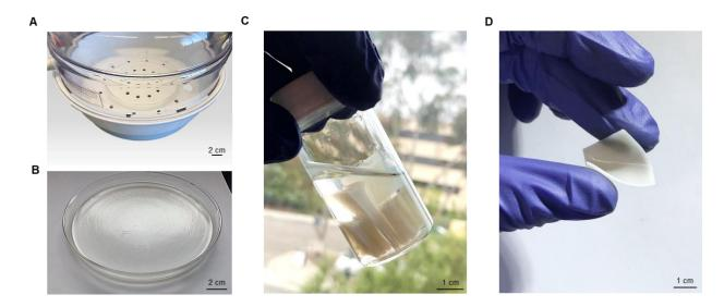
**Supplementary Figure 4**. Images of the fabrication of the KOH-PVA electrolyte gel. (A) Drying of the precursor solution to desired concentration in a vacuum desiccator. (B) The crosslinked 36.5 % hydrogel after drying. (C) Storage of the hydrogel pieces after cutting into desired sizes. (D) A bent  $2 \times 2$  cm<sup>2</sup> hydrogel.
