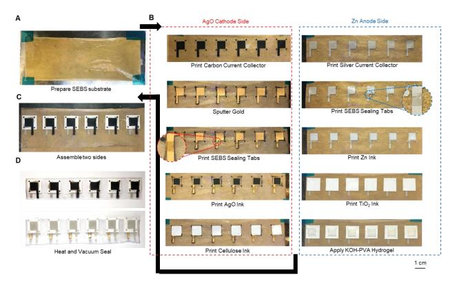
**Supplementary Figure 2**. The images of the step-by-step batched fabrication of the printed AgO-Zn batteries. (A) Prepared SEBS substrate. (B) The layer-by-layer printing of the AgO cathode (left) and the Zn anode (right). (C) Placing the cathode side onto the anode side with the hydrogel electrolyte in between. (D) Heat and vacuum sealing of the batteries. Each cell was separated by further heat sealing after the entire batch was vacuum sealed.
