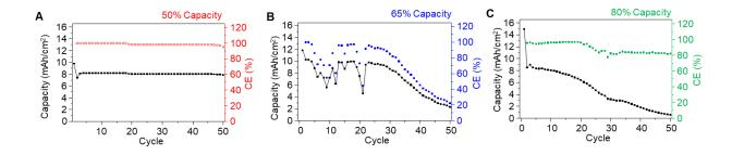
**Supplementary Figure 12.** The cycling of the battery at the different capacity range. (A) Cycling the battery between 40 % and 9 0% state of charge (50 %). (B) Cycling the battery between 2 5% and 90 % state of charge (65 %). (C) Cycling the battery between 10 % and 90 % state of charge (80 %). Electrolyte with the concentration of 36.5 % was used, and the cells were cycled at the rate of 0.2 C.
