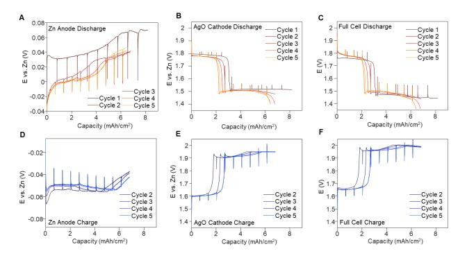
**Supplementary Figure 18**. The potential profile of the anode (A,D) and cathode (B,E) vs. Zn reference and the full cell (C, F) within the first 5 cycles of (A-D) discharging and (D-F) corresponding 4 cycles of charging. The vertical lines correspond to the places where an EIS measurements were taken.
