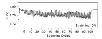
**Supplementary Figure 20**. The voltage profile of the  $1 \times 5$  cm<sup>2</sup> battery during 1 mA discharge while undergoing 100 cycles of 10 % lengthwise stretching. Although the battery was not optimized for stretchability, a certain amount of stretchability is required for the battery to endure low-radius bending and accommodate for the outer-layer strain.
