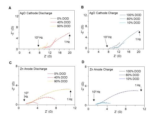
**Supplementary Figure 17**. The Nyquist plot and the EIS fitting of the cathode during the 5<sup>th</sup> cycle (A) discharging and (B) charging, and the corresponding anode (C) charging and (D) discharging.
