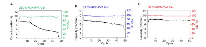
**Supplementary Figure 13**. The cycling of the battery with electrolyte concentration of (A) 26.3 %, (B) 31.8 %, and (C) 36.5 %. The 50 % capacity range was used and the cells were cycled at the rate of 0.2 C.
