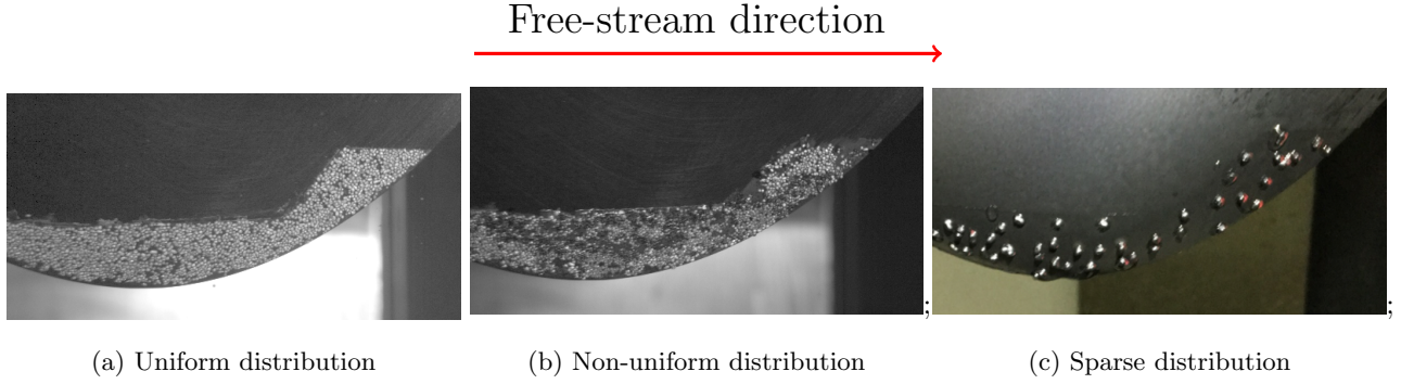
Fig. 4: Different distributions of sand grains for the roughness pattern (II).
