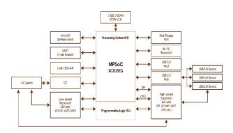
[13, Fig. 5] : Block Diagram of Ultra96 Block diagram
