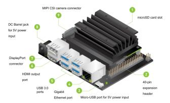
[Fig. 6] Block Diagram of Nvidia Jetson Nano
